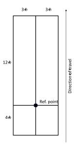
**Figure 2.** Dimension of the boundary area for  $Q_0$  calculation where h is the installation height of the luminaire.
