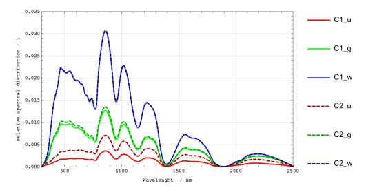
**Figure 6.** Spectral distribution in the 300–2500 nm wavelength range of the solar radiation reflected by the cores (see Table 1) considering the measured values of reflectance in laboratory conditions (8/d geometry).
