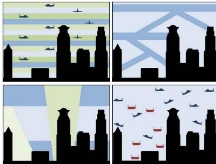
**Figure 11.** Metropolis airspace concepts Layers, Tubes, Zones and Full Mix [50].
