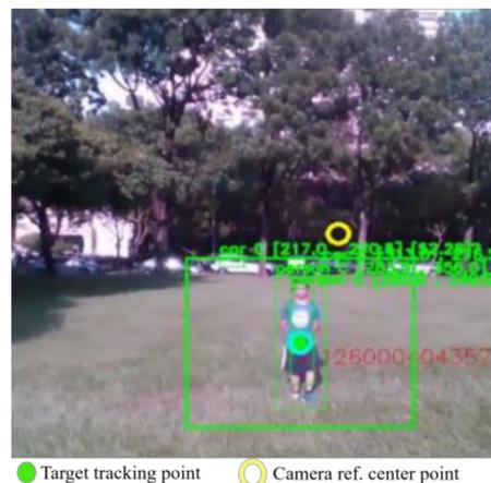
Figure 20. Front tracking of the target from the view of the quadcopter.
