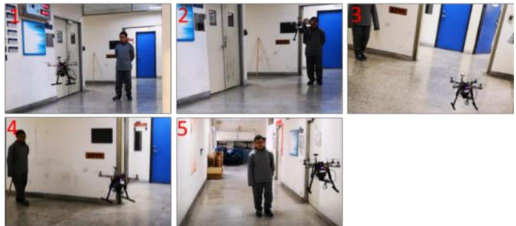
**Figure 23.** UAV tracking target test at the corridor (The sequence of target movement and UAV tracking is shown in 1–5).
