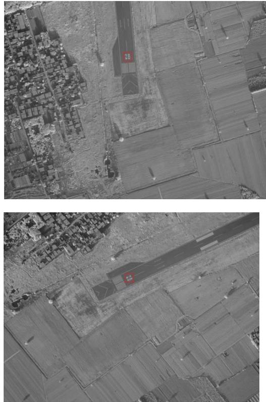
**Figure 14.** The ground images captured by two drones at the same time, with the number “28” in the red box as the ground identifier, and their true coordinates are known.
