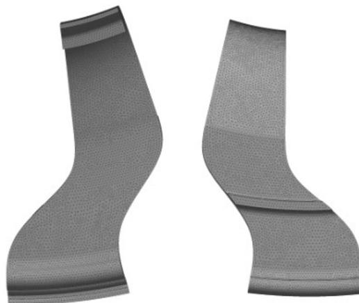
Figure 12. The mesh structure of the turbine stationary blade.
