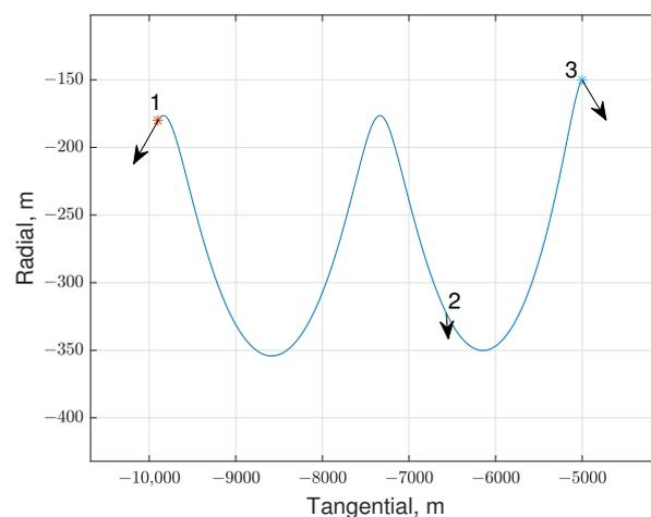
**Figure 3.** Relative 2D Path in Hill's Coordinates.
