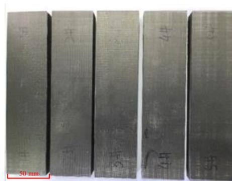
Figure 7. Photograph of 3-points bending specimens.
