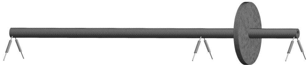
**Figure 29.** Finite element model and constraints of the LP turbine.
