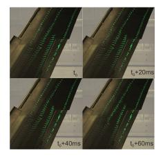
Figure 10. Progression of separation on the inboard section.
