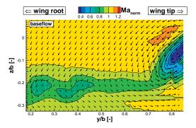
**Figure 21.** Wake flow at  $(\alpha_{max,base} + 0.7^{\circ})$  for the base flow.
