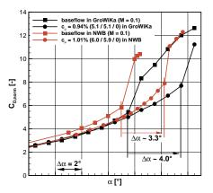
**Figure 5.** Comparison of results obtained in the GroWiKa wind tunnel [18] and the NWB wind tunnel at M = 0.1.
