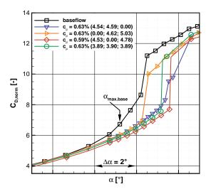
**Figure 11.** Drag coefficient for forcing with  $c_{\mu} \approx 0.6\%$ .
