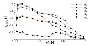
Figure 8. Pressure coefficient curve in the spanwise direction for various incidence angles.
