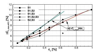
Figure 18. Maximum lift increase for different momentum coefficients and segment combinations.
