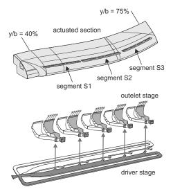
Figure 2. Sketch of the active flow control (AFC) system.
