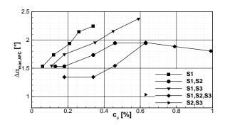
Figure 16. Stall angle offset for different momentum coefficients and segment combinations.
