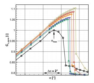
**Figure 15.** Lift coefficient for forcing with Segments 1 and 3 for various  $c_{\mu}$ ; see Figure 14 for the line legend.
