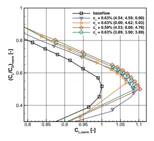
**Figure 13.** Aerodynamic efficiency vs. lift coefficient for forcing with  $c_{\mu} \approx 0.6\%$ .
