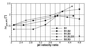
Figure 17. Stall angle offset for different velocity ratios and segment combinations.
