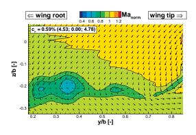
**Figure 22.** Wake flow at ( $\alpha_{max,base} + 0.7^{\circ}$ ) for the controlled flow.
