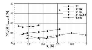
**Figure 19.** Drag reduction at  $\alpha_{max,AFC}$  for different momentum coefficients and segment combinations.
