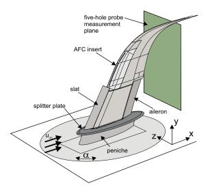
Figure 1. Sketch of wind tunnel model.
