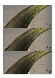
Figure 9. Progression of separation on the outboard section.
