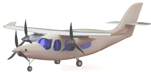
Figure 4. Conceptual prototype “Skybrid” hybrid electric skydiving/freight aircraft.
