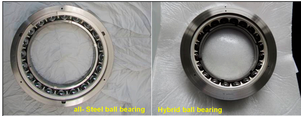
Figure 2. Pictures of the tested bearings. The hybrid version incorporates Squeeze film damping as an additional feature.
