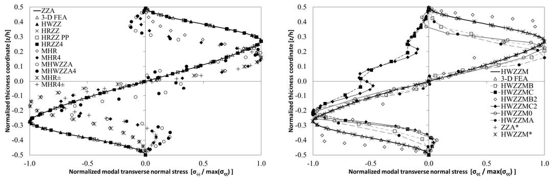
Figure 7. Case c1: Normalized modal displacements and stresses of a simply supported laminated plate ( $Lx/h = 5, E_1/E_2 = 40$ ).
