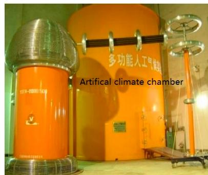
**Figure 4.** Artificial icing test.
