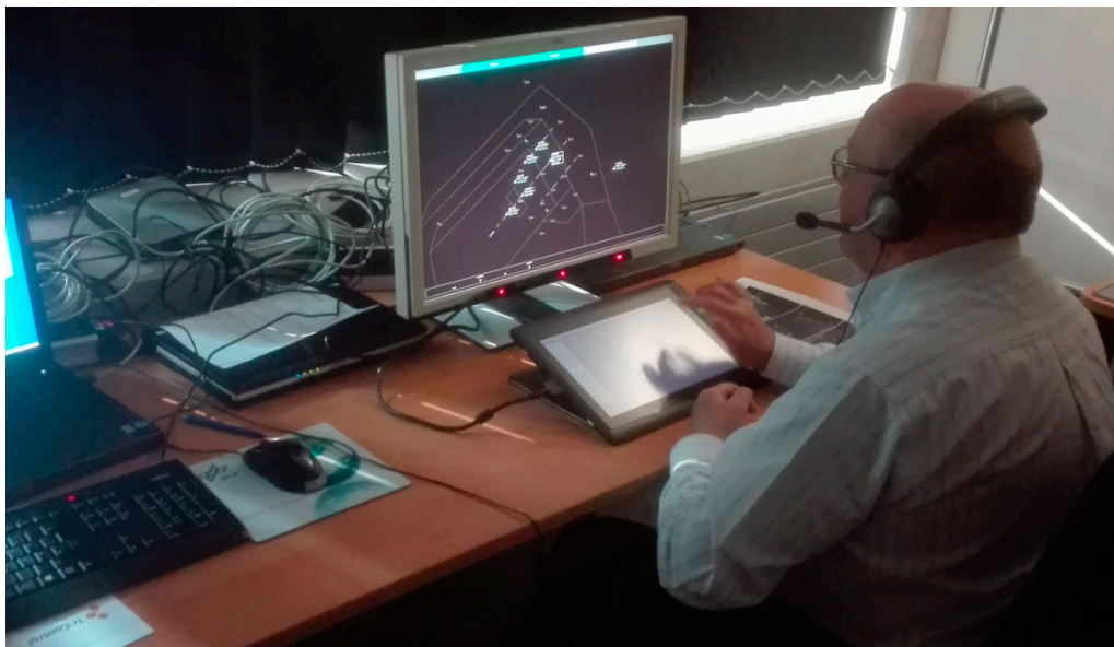
Figure 3. Setup of TriControl feasibility simulation study with a participant before uttering a command value, after performing a command type gesture and selecting an aircraft with his eyes.
