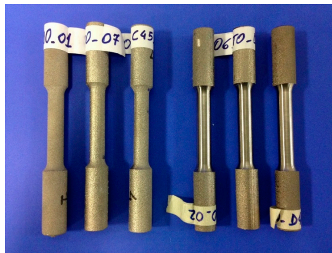
Figure 3. Three as built (on the left side) and three machined specimens after EBM process (on the right side).
