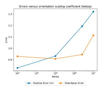
**Figure 7.** Experimental results from varying the orientation scaling coefficient in the exponential-based model.
