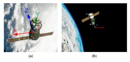
Figure 3. (a) Axis notation for a moving spacecraft frame, and (b) axis notation of the camera frame.
