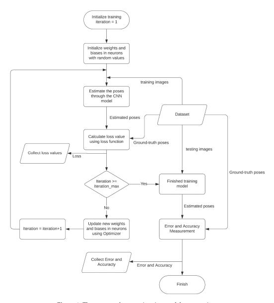
**Figure 1.** The process of pose estimation model construction.
