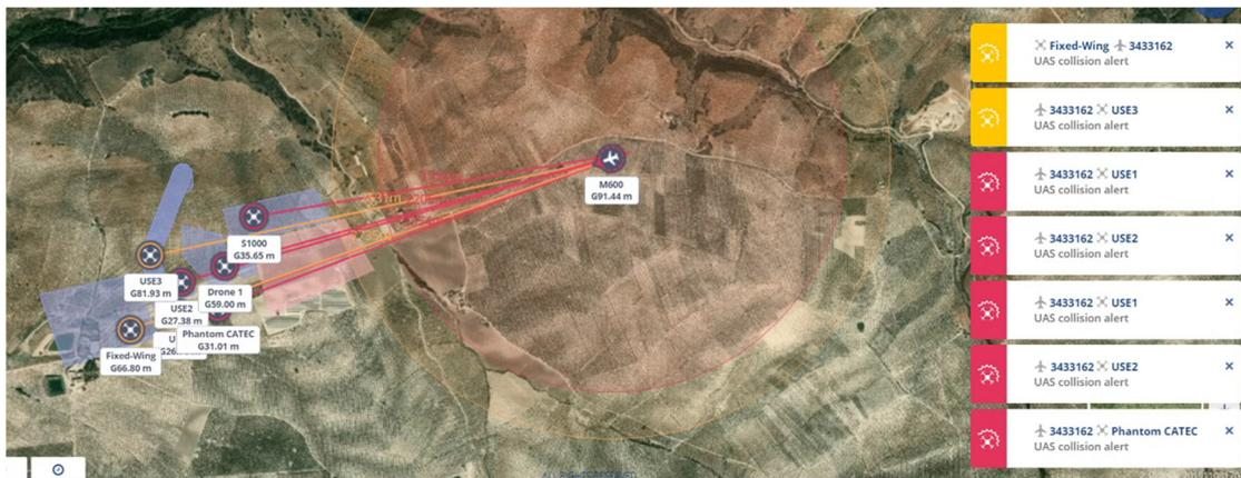
Figure 13. Seven drones flying simultaneously with a general aircraft in VLL in an emergency situation.
