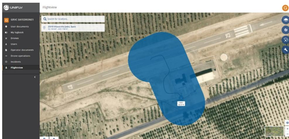
**Figure 17.** Image from Unifly USP showing the final trajectory performed by the drone and the whole area reserved in the U-space system.
