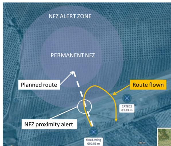
Figure 8. NFZ alert distance scenario showing the key elements.
