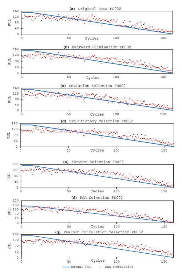
Figure 13. (a–g) RUL prediction points for one engine of FD002 test data.
