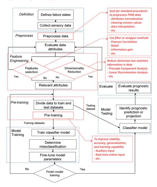
Figure 4. The prognostic data-driven framework for neural network algorithms.
