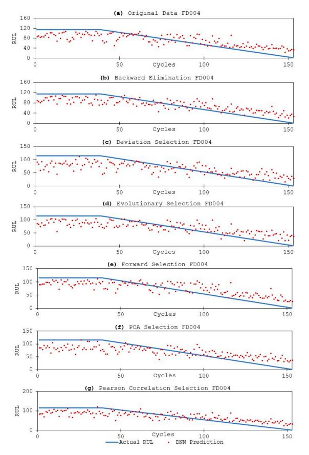
Figure 14. (a–g) RUL prediction points for one engine of FD004 test data.
