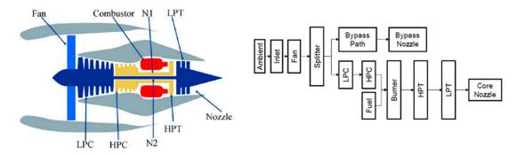
Figure 5. Engine and sensor points (left) and engine parts modules connections (right) [39].
