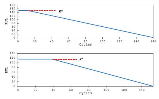
Figure 9. Example of RUL curve of one testing engine: FD002 (top) and FD004 (bottom).
