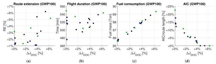
**Figure 5.** The plots show trajectory data of the Pareto-optimal solutions for the environmental cost function based on GWP<sub>100</sub>: (a) route extension with respect to the great circle distance between WP1 and WP2; (b) flight duration; (c) fuel consumption; (d) fraction of AIC length with respect to route length, plotted against  $\Delta J_{DOC}$ . Green dots represent trajectories plotted in Figure 4.
