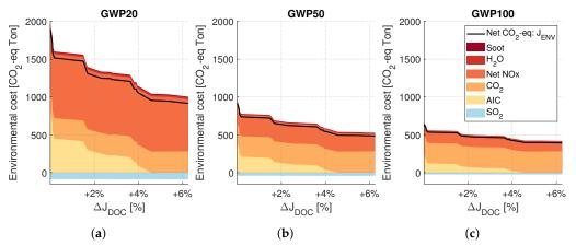
**Figure 3.** Individual climate forcing components of the environmental cost  $J_{ENV}$ , expressed in  $CO_2$ -equivalent Ton, for environmental cost function based on: (a)  $GWP_{20}$ , (b)  $GWP_{50}$ , (c)  $GWP_{100}$ . Negative values for  $SO_2$  indicate a cooling forcing.
