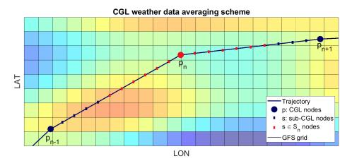
**Figure 1.** Scheme of the averaging method used to pass along-trajectory weather information to the CGL nodes p of the optimization algorithms. The number of sub-CGL nodes s is chosen to have a spatial resolution similar to the GFS grid with weather data. The gradient color map represents different values of a generic GFS data variable.
