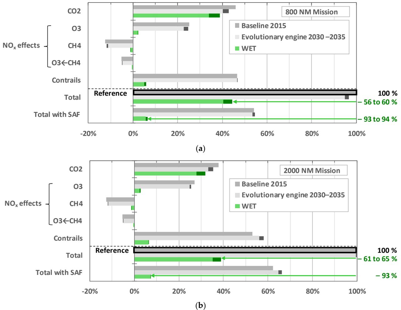
**Figure 2.** Absolute Global Warming Potentials over one hundred years relative to the total of the Baseline 2015 reference aircraft on missions of (a) 800 NM, (b) 2000 NM. “Contrails” includes contrail cirrus by applying a multiplier of 5 on the line-shaped results. Ranges are given as range of the SFC reduction potential. No scientific uncertainties concerning the climate impacts are issued.
