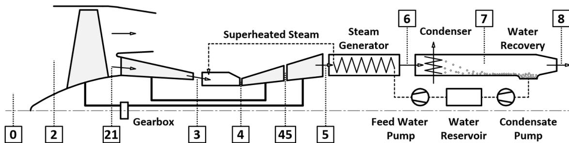
**Figure 1.** Scheme of a half-side arrangement of the proposed water-enhanced turbfan concept with station nomenclature (taken from [11]).
