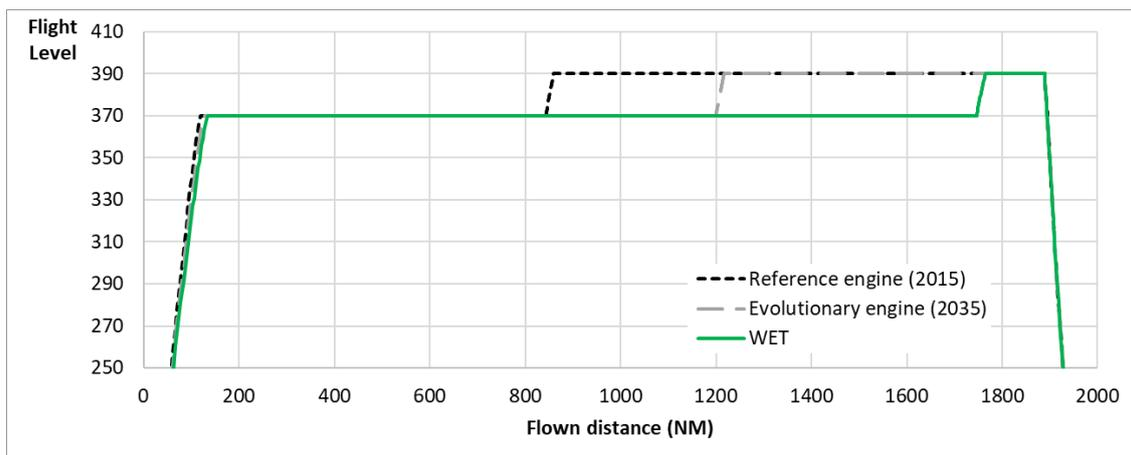
**Figure 3.** Mission paths of the three different aircraft concepts, for upper-end SFC reduction potentials.
