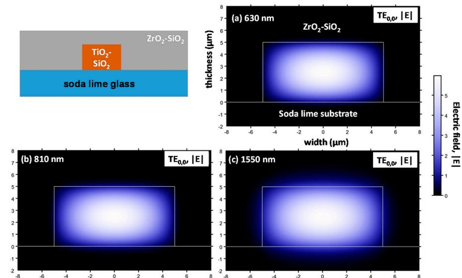
**Figure 13.** Simulated  $TE_{00}$  mode of a  $TiO_2$ – $SiO_2$  waveguide deposited on soda-lime glass and surrounded by the  $ZrO_2$ – $SiO_2$  cladding and operating at (a) 630 nm, (b) 810 nm and (c) 1550 nm. The thicknesses and widths are 5  $\mu m$  and 10  $\mu m$ , respectively.
