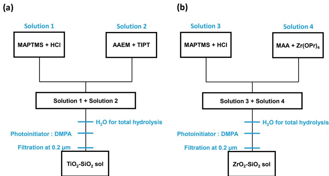
**Figure 2.** Preparation of the different organic–inorganic sol–gel solutions. Material synthesis of (a) TiO<sub>2</sub>–SiO<sub>2</sub> and (b) ZrO<sub>2</sub>–SiO<sub>2</sub> sols. In both cases, a photoinitiator (DMPA) is added to induce the start of UV-polymerization reactions.
