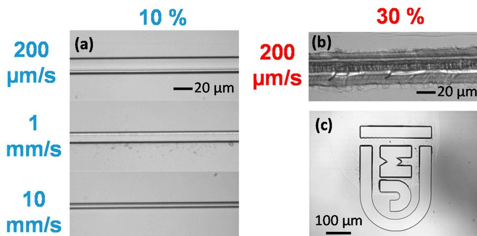
**Figure 7.** Structures obtained by the direct writing technique showing (a) lines obtained at 10% and for different scanning speed ( $200\ \mu\text{m/s}$ , 1 and  $10\ \text{mm/s}$ ), (b) calcinated trace induced at 30% and  $200\ \mu\text{m/s}$  and (c) Jean Monnet University logo with a  $420\ \mu\text{m}$  size in height.
