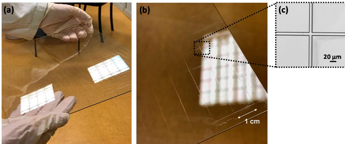
**Figure 9.**  $\text{TiO}_2\text{-SiO}_2$  grid architecture on a large substrate composed of 62 guides. (a) Overview of the sensor, (b) corresponding zoom showing the 1 cm separation between two consecutive lines and (c) microscope image of the doubled exposed zone.
