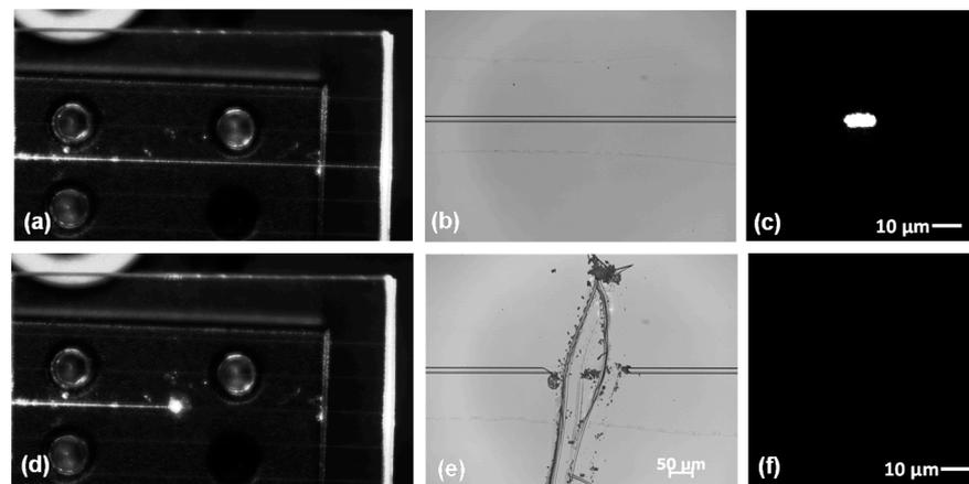
**Figure 16.** Damage detection with a  $\text{TiO}_2\text{-SiO}_2$  waveguide operating at 638 nm showing: (a) top-view of the unaffected guide before the impact, (b) corresponding microscope image and (c) guided mode. After the impact: (d) top-view, (e) microscope image and (f) absence mode observation.
