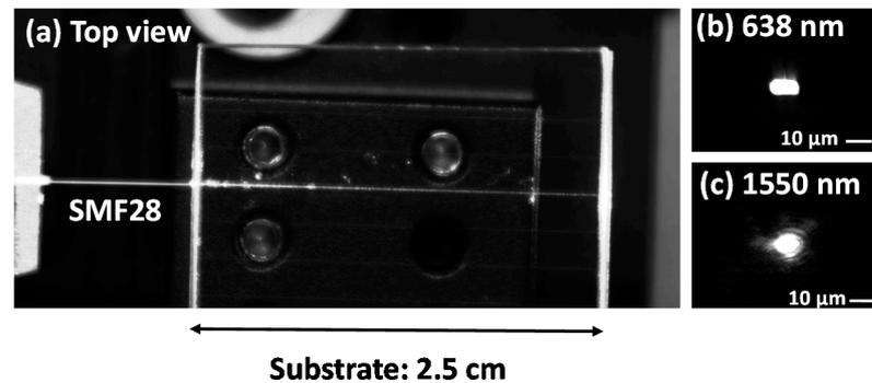
**Figure 14.** Characterization of TiO<sub>2</sub>-SiO<sub>2</sub> waveguides (surrounded by air). The figure illustrates: (a) top-view of the waveguide injection at 638 nm, (b) output optical guided mode at 638 nm and (c) guided mode at 1550 nm.
