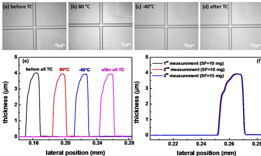
**Figure 19.** Thermal cycling (TC) effect on a TiO<sub>2</sub>–SiO<sub>2</sub> grid architecture. Microscope images of the grid area are given (a) before the thermal cycling, (b) after being thermally treated at 80 °C, (c) –40 °C and (d) after all the consecutive thermal treatments. (e) Corresponding profilometer measurements (SF = 10 mg) and (f) profilometer measurements of the structure submitted to the full thermal cycling with SF of 10 mg (black and red lines) and 15 mg (blue line).
