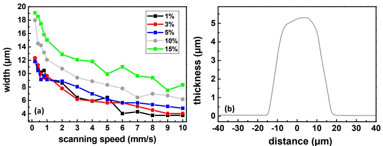
**Figure 8.** Characterization of the photo-induced patterns using the Dilase 750 facility. (a) Width of the structures as a function of the scanning speed for powers ranging from 1% and 15% and (b) profile obtained for a line written at 10% and 200  $\mu\text{m/s}$ .
