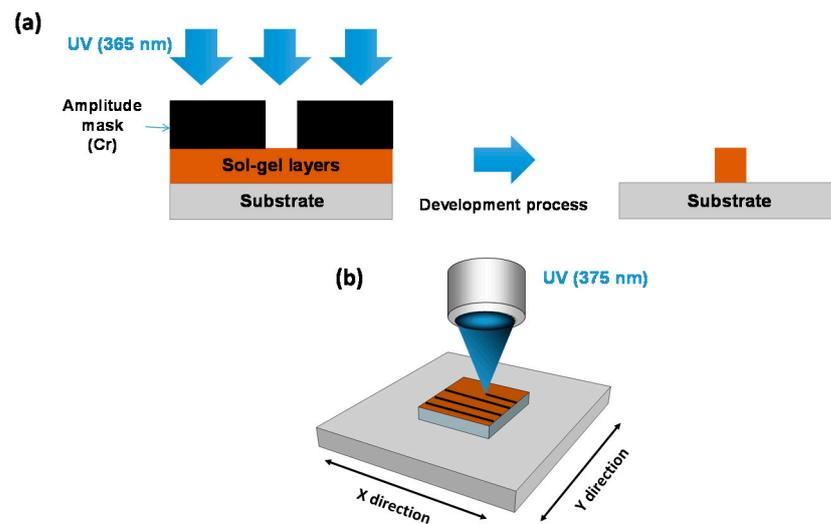
**Figure 3.** Example of the photolithography processes used for the layer structuration. (a) Photolithography by photomask on an organic–inorganic layer. (b) Principle of the direct writing technique (Dilase 750 from Kloé company, Montpellier, France). A laser beam is focused on the hybrid thin films. The structures are created by the translation of the stages in the X and Y directions while the laser beam is fixed. The black lines on the layer represent the UV photopolymerized exposed regions.
