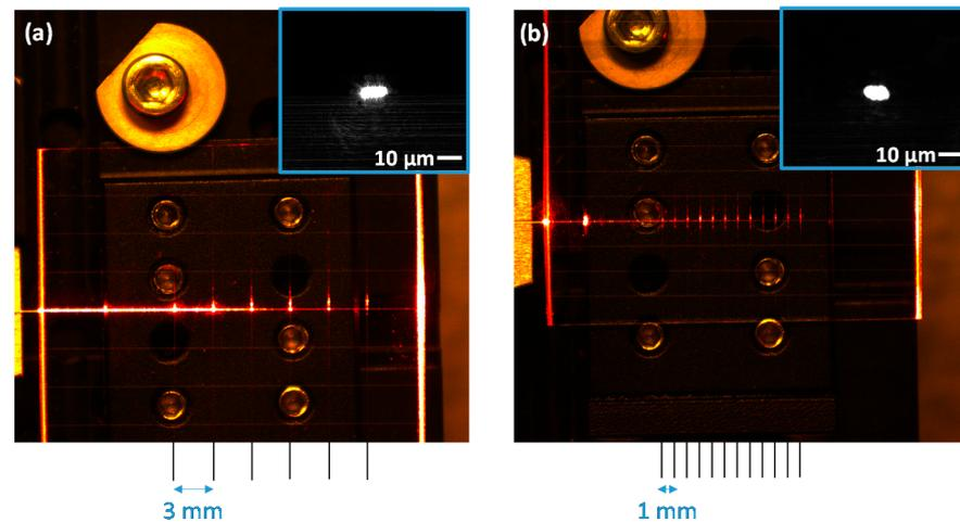
**Figure 17.** Top-view of  $\text{TiO}_2\text{-SiO}_2$  waveguide grid after signal injection at 638 nm for (a) 6 perpendicular waveguides spaced by 3 mm and (b) 12 perpendicular waveguides spaced by 1 mm. In both cases, the corresponding inset illustrates the guided mode at 638 nm, and the waveguides are surrounded by air.
