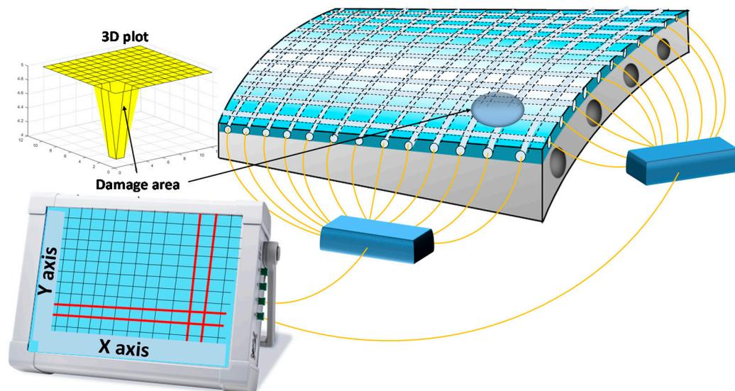
**Figure 1.** Final architecture of the 2D sol-gel matrix sensor for damage detection. The sensor is based on a grid of optical waveguides. An impact on the plane leads to the degradation or the rupture of one or more waveguides. Thanks to the particular 2D structure of the sensing material, the identification of the impacted damage allows the damage localization.
