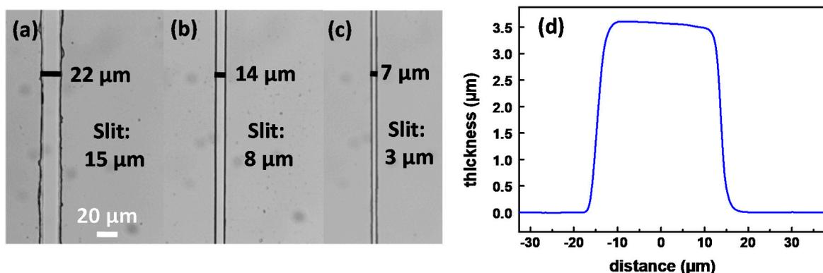
**Figure 4.** TiO<sub>2</sub>–SiO<sub>2</sub> patterns obtained using the amplitude mask with different slits at 15 μm, 8 μm and 3 μm. Microscope observations (reflection ×20) of (a) line obtained with a slit of 15 μm in width, (b) line obtained with a slit of 8 μm and (c) line obtained with a slit of 3 μm. (d) Profilometer measurement of (a).
