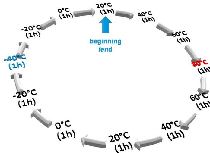
**Figure 18.** Thermal cycling performed on a 10 cm × 10 cm TiO<sub>2</sub>–SiO<sub>2</sub> grid architecture divided into three steps: a first increase from 20 °C to 80 °C followed by a decrease down to –40 °C, while the last increase is performed to reach 20 °C. Each temperature level lasts 1 h.
