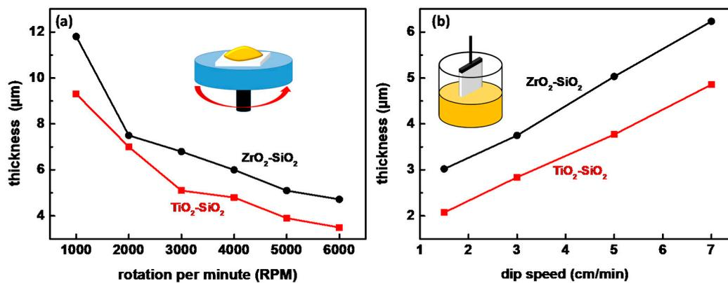
**Figure 5.** Investigation of  $\text{TiO}_2\text{-SiO}_2$  (red squared curve) and  $\text{ZrO}_2\text{-SiO}_2$  (black dotted curve) thicknesses using the spin coating (a) and the dip coating (b) methods.
