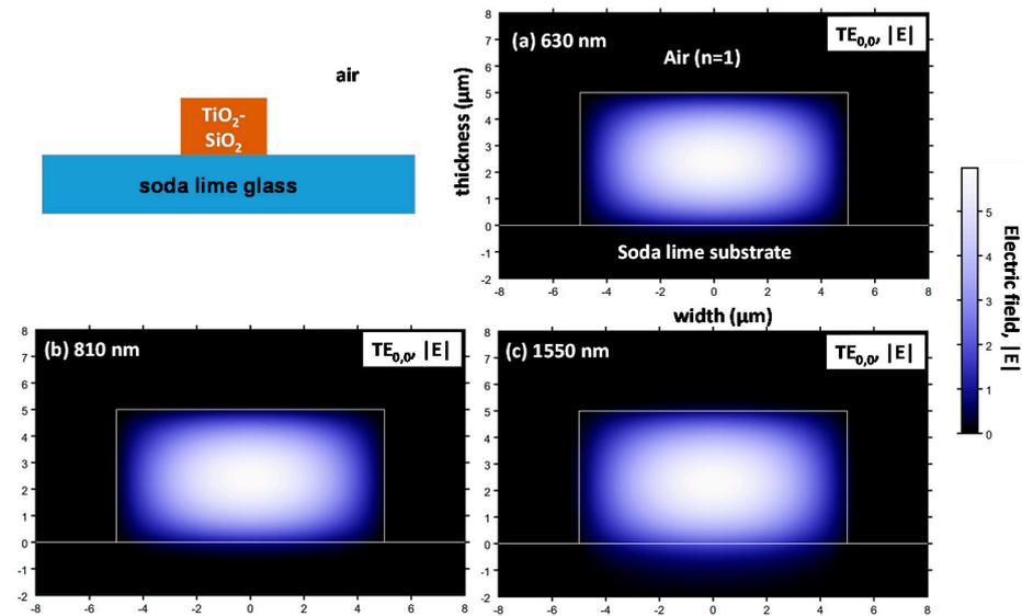
**Figure 12.** Simulated transverse electric  $TE_{00}$  mode of a  $TiO_2$ - $SiO_2$  waveguide deposited on a soda-lime glass surrounded by air and operating at (a) 630 nm, (b) 810 nm and (c) 1550 nm. The thicknesses and widths are 5  $\mu\text{m}$  and 10  $\mu\text{m}$ , respectively.
