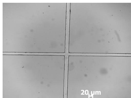
**Figure 6.**  $\text{TiO}_2\text{-SiO}_2$  grid observed using an optical microscope in a reflection mode ( $\times 20$ ). The crossed  $\text{TiO}_2\text{-SiO}_2$  area is not affected by the double exposure (360  $\text{J}/\text{cm}^2$ ).
