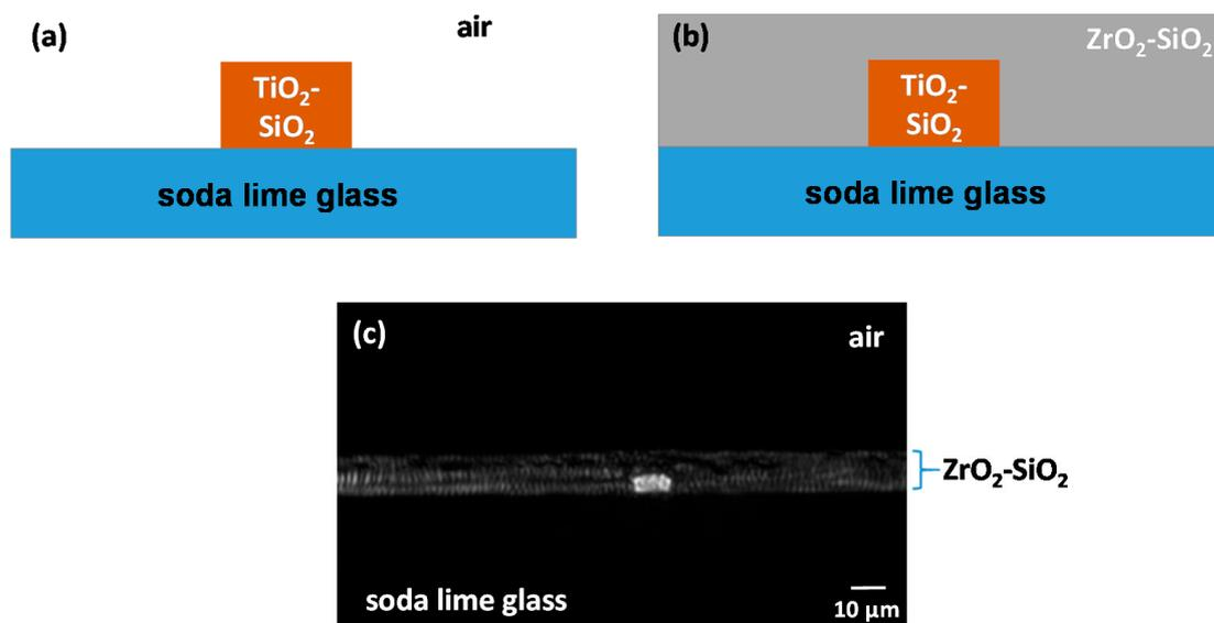
**Figure 10.** Two configurations of the photonic device deposited on soda-lime glass. (a)  $\text{TiO}_2\text{-SiO}_2$  core without cladding and surrounded by air. (b)  $\text{TiO}_2\text{-SiO}_2$  core buried in a  $\text{ZrO}_2\text{-SiO}_2$  coating and (c) output light of the  $\text{TiO}_2\text{-SiO}_2$  core waveguide with  $\text{ZrO}_2\text{-SiO}_2$  cladding obtained experimentally.
