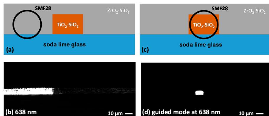
**Figure 15.** Injection of visible light (638 nm) in the architecture composed of the TiO<sub>2</sub>-SiO<sub>2</sub> core deposited on soda-lime glass and surrounded by the ZrO<sub>2</sub>-SiO<sub>2</sub> cladding. (a) Diagram of the SMF28 misaligned with the core, (b) corresponding output, (c) diagram of SMF28 aligned with the core and (d) corresponding guided mode. The SMF28 is schematized by black circles.
