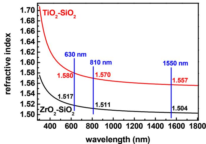
**Figure 11.** Refractive index of  $\text{TiO}_2\text{-SiO}_2$  (red line) and  $\text{ZrO}_2\text{-SiO}_2$  (black line) obtained by the ellipsometry technique. The layers were insolated by UV photons and thermally treated.
