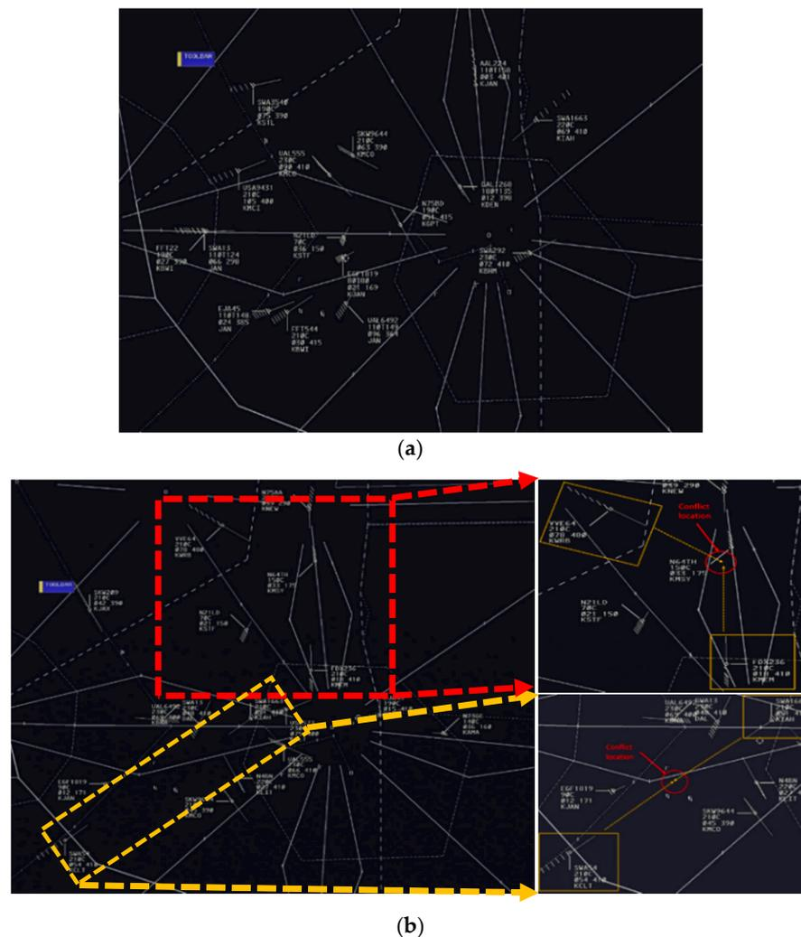
**Figure 2.** Example scenarios: (a) Layout of aircraft during an experiment using one of the scenarios; (b) Example of aircraft conflicts highlighted in red and yellow (left side shows the aircraft layout at a certain point in time, and the right side shows the future conflict locations).
