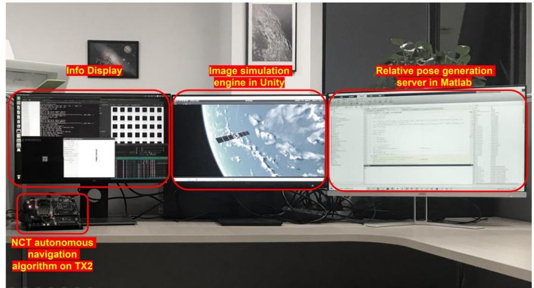
Figure 10. Hardware-in-the-loop (HIL) simulation platform.
