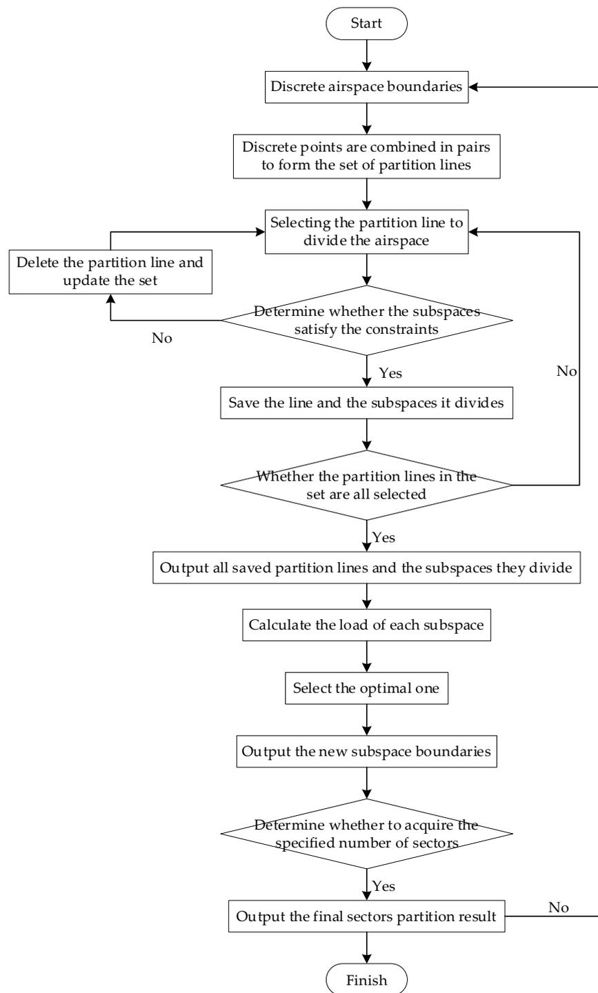
Figure 3. BSP algorithm flow chart.
