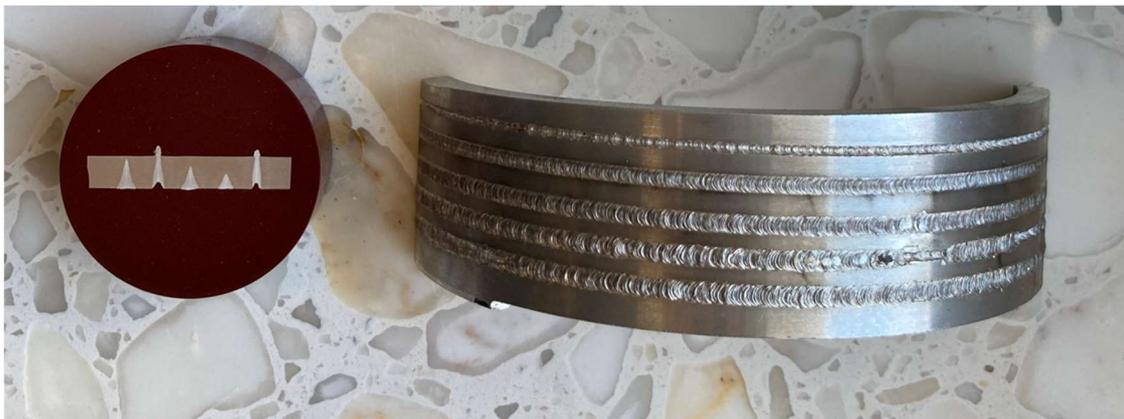
**Figure 6.** Aluminium alloy electron beam welding trial.
