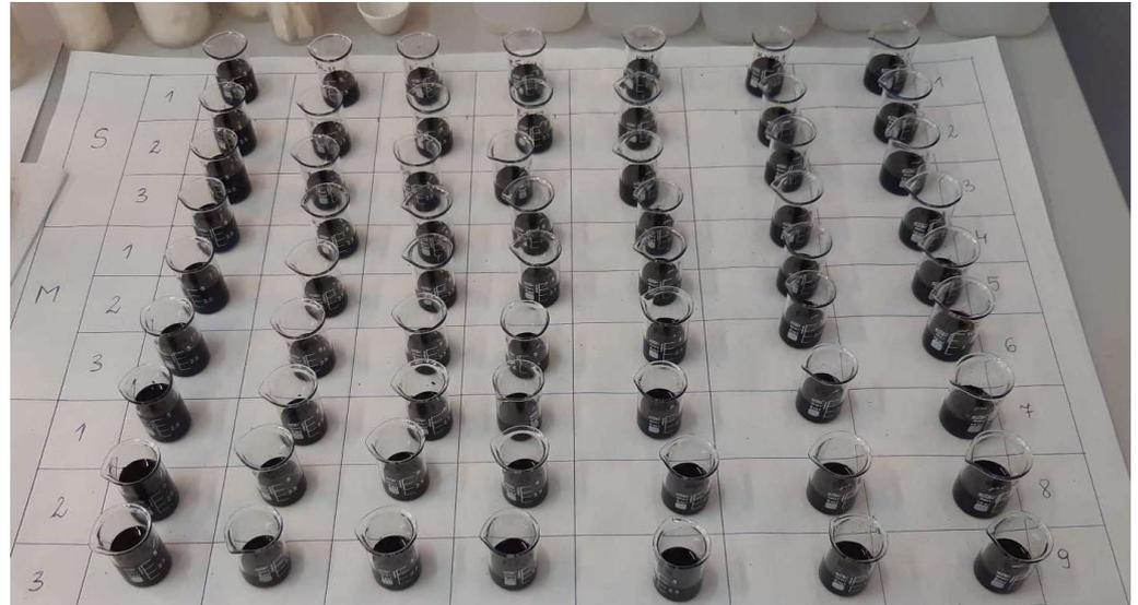
**Figure 3.** Preparation of  $Mn_2O_3/Al_2O_3$  catalyst bed at L-IoA for initial screening.
