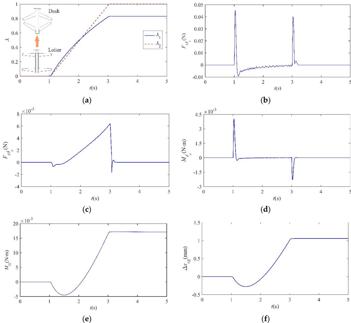
**Figure 4.** The open-loop dynamic responses of transition process from loitering configuration to dashing configuration. (a) The variation ratios during transition process; (b)  $F_{x\delta}$ , (c)  $F_{z\delta}$ , (d)  $M_\delta$ , (e)  $M_G$ , (f) Shift of gravity center,  $\Delta x_{cg}$ .
