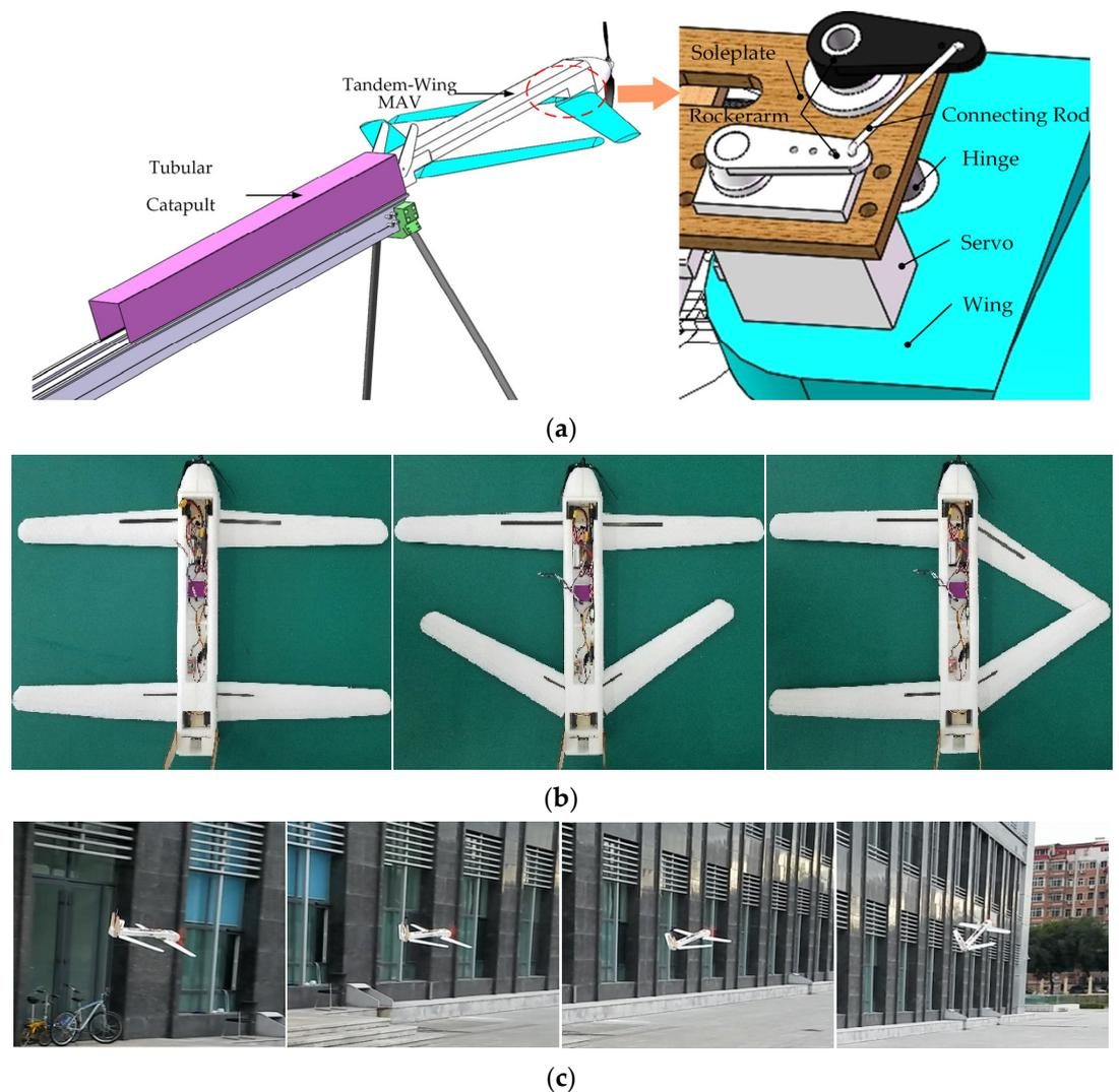
**Figure 1.** Schematic diagram and prototype of the multitask tandem-wing MAV with variable sweep. (a) Schematic diagram of the sweep morphing; (b) Prototype of the tandem-wing MAV in different variable sweep configurations: no-sweep configuration, symmetric sweep morphing, asymmetric sweep morphing; (c) Flight test of symmetric morphing for pitch control.
