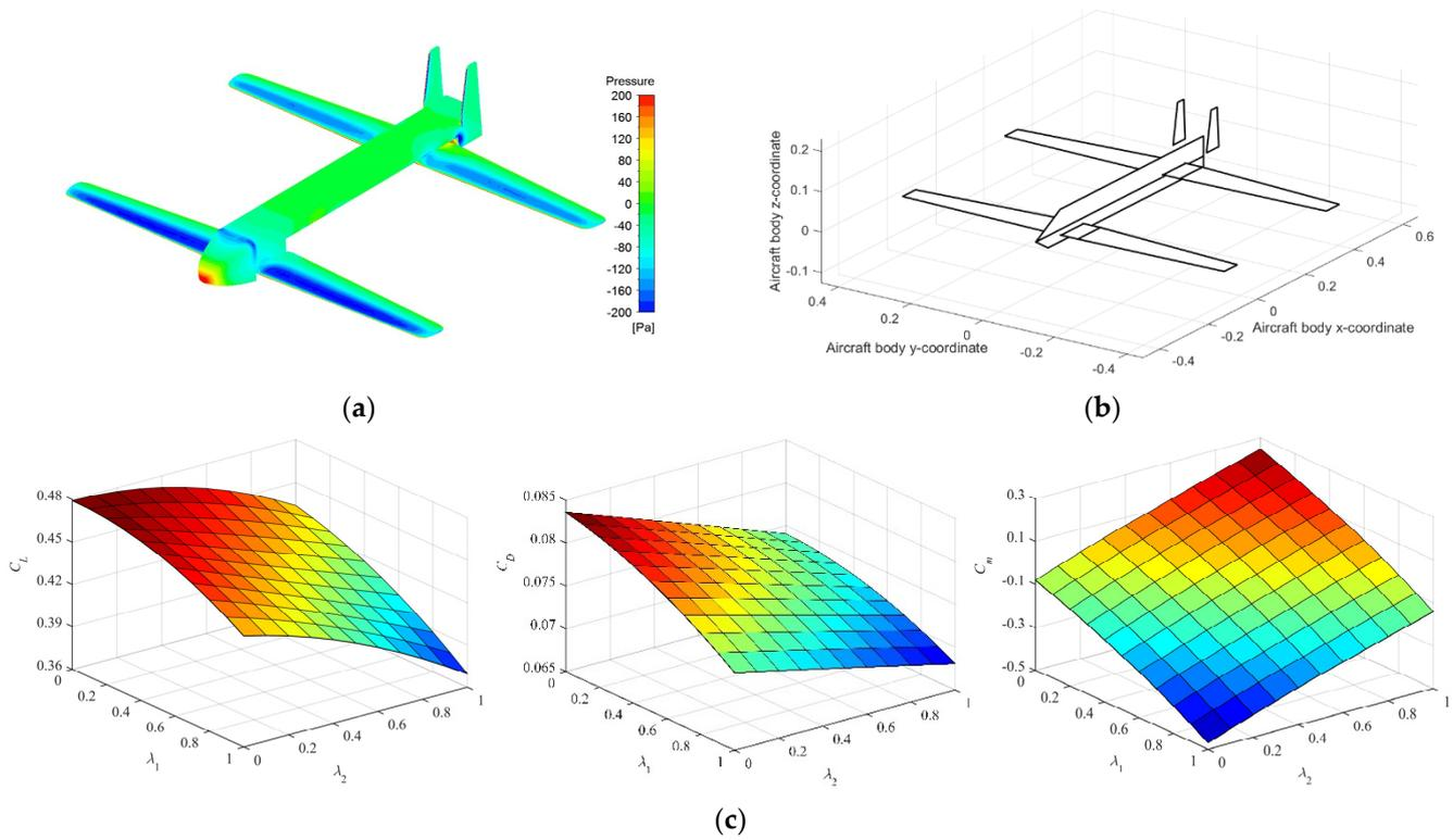
**Figure 3.** Aerodynamic characteristics acquired by CFD and VLM. (a) Pressure distribution on the MAV with the CFD approach; (b) The MAV configuration in VLM; (c) Aerodynamic coefficients under different variation ratios ( $\alpha = 4^\circ$ ): lift coefficient, drag coefficient, pitch moment coefficient.
