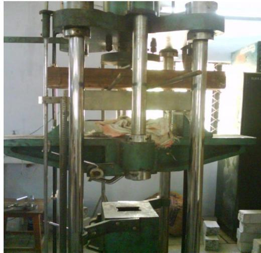
**Figure 2.** Flexural strength testing setup.
