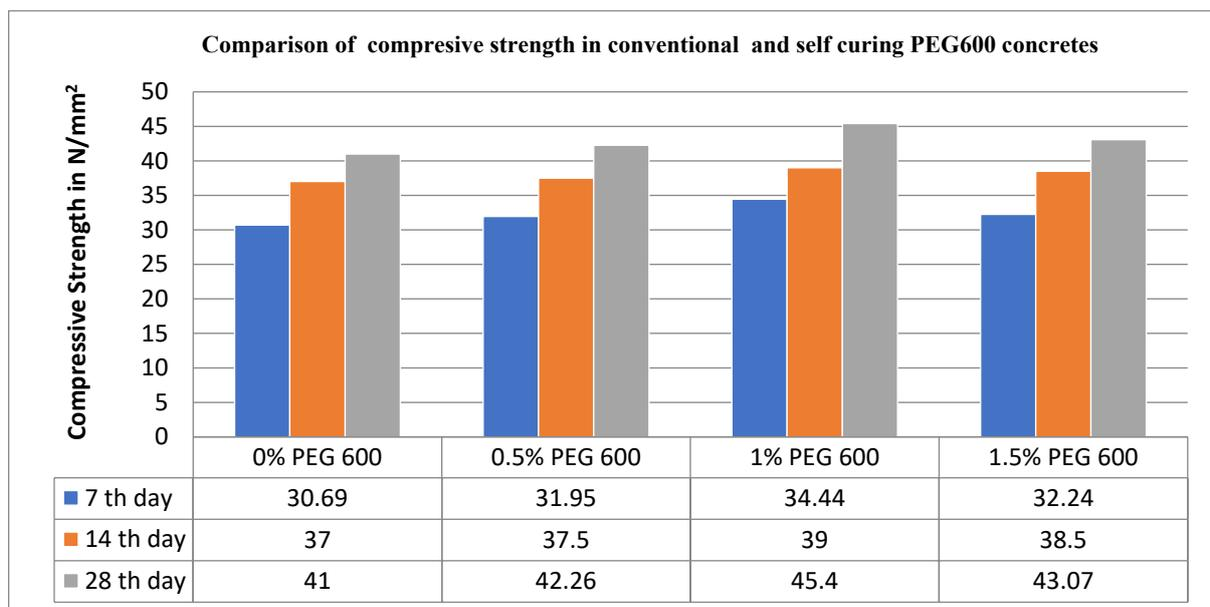
**Figure 4.** Comparison of compressive strength in conventional and PEG-600 concretes.
