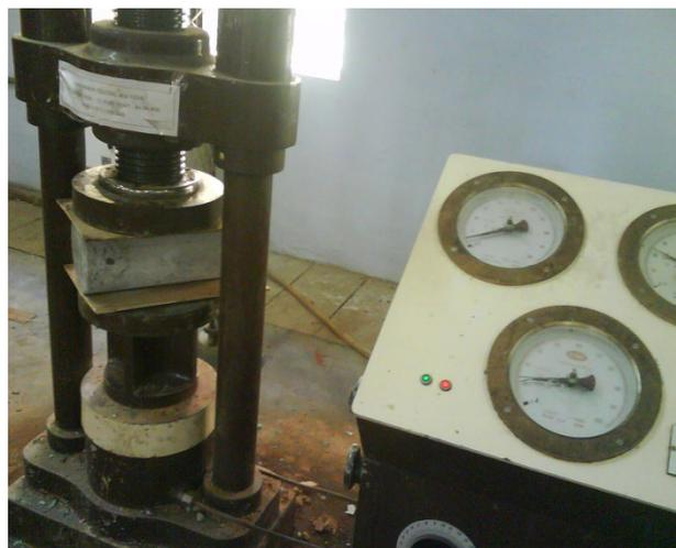
**Figure 3.** Split tensile test setup.
