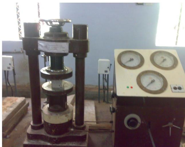
**Figure 1.** Compressive Strength Test setup.
