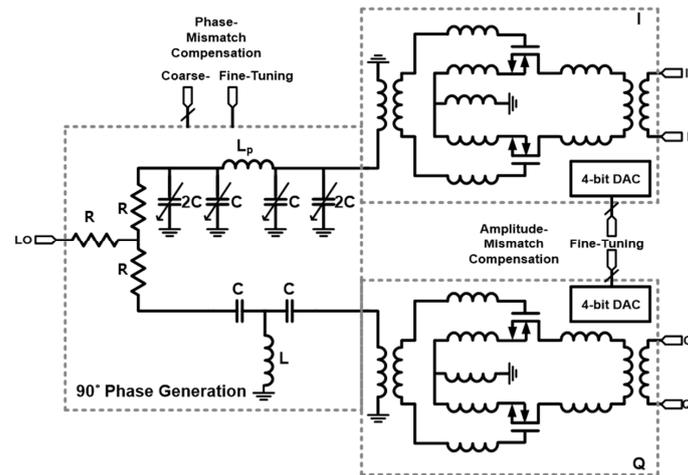
**Figure 3.** Schematic of a quadrature generator.
