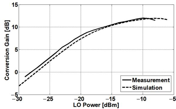
**Figure 9.** Measured and simulated conversion gain of mixer with respect to LO power:  $f_{LO} = 28$  GHz;  $f_{IF} = 400$  MHz;  $P_{IF} = -30$  dBm.
