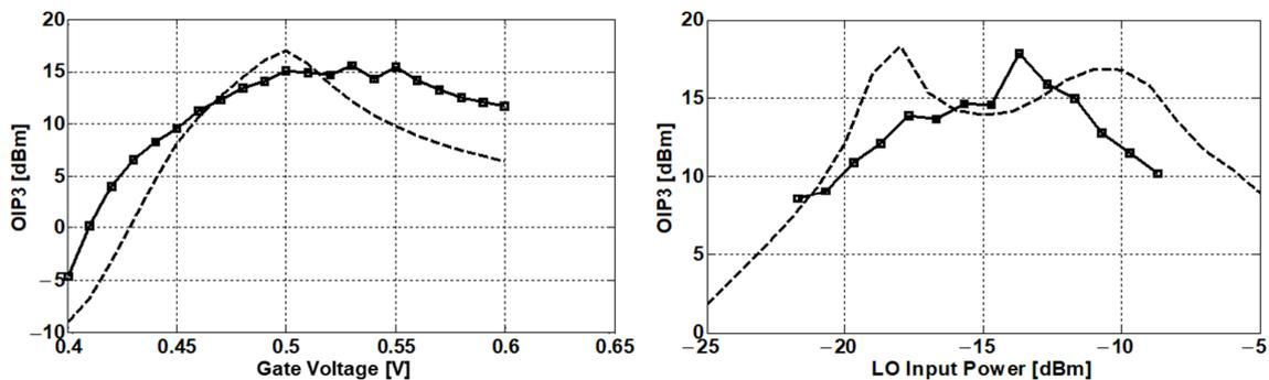
**Figure 11.** Simulated and measured OIP3 of mixer.
