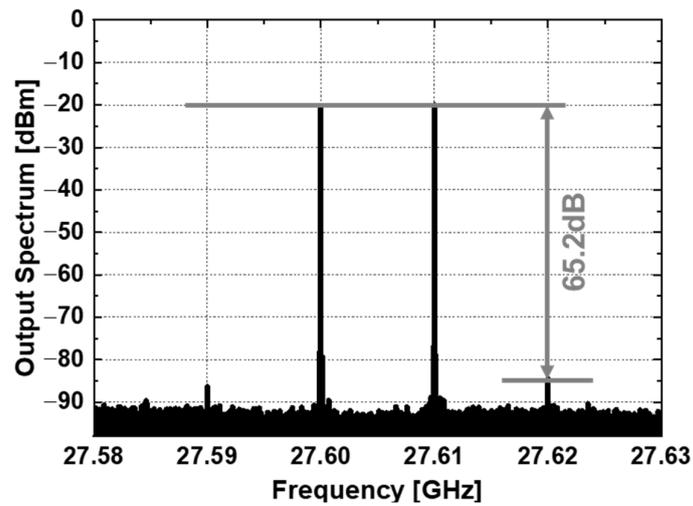
Figure 12. Measured output spectrum for OIP3:  $f_{LO} = 28$  GHz;  $f_{IF1} = 390$  MHz;  $f_{IF2} = 400$  MHz.
