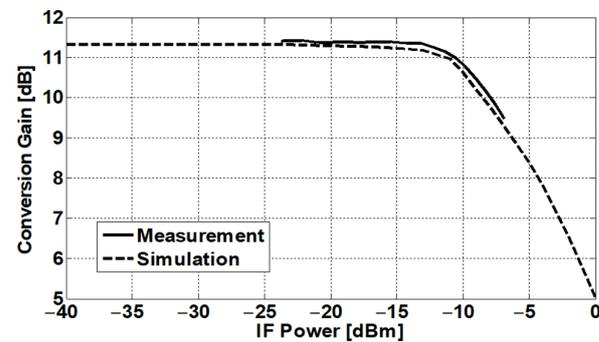
**Figure 10.** Measured and simulated conversion gain of mixer with respect to IF power:  $f_{LO} = 28$  GHz;  $f_{IF} = 400$  MHz;  $P_{LO} = -13$  dBm.
