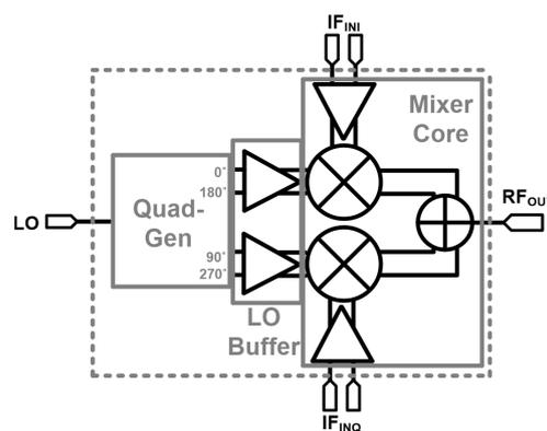
Figure 2. Block diagram of the fabricated I/Q up-conversion mixer.
