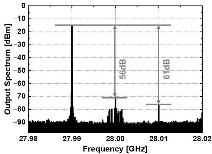
Figure 13. Measured output spectrum for LO leakage and IRR:  $f_{LO} = 28$  GHz;  $f_{IF} = 10$  MHz;  $P_{LO} = -13$  dBm.
