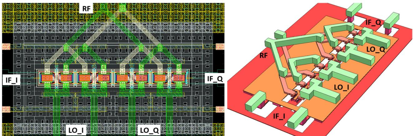
**Figure 5.** Two- and three-dimensional layout of switching stage.
