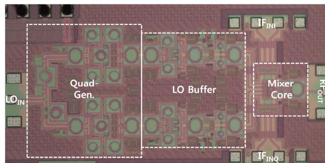
Figure 6. Chip microphotograph of proposed up-conversion mixer.
