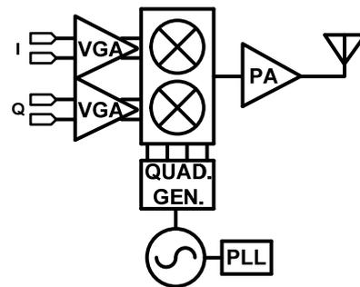
Figure 1. Block diagram of a direct up-conversion mm-wave transmitter.
