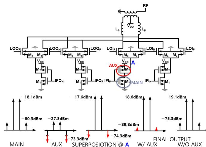
**Figure 4.** Schematic of mixer core and intermodulation components in the two-tone test.
