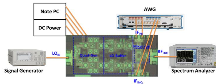
Figure 7. Measurement setup for CG, P1dB and OIP3.
