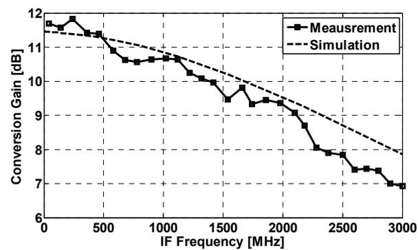
Figure 8. Simulated and measured mixer conversion gain versus IF frequency:  $f_{LO} = 28$  GHz;  $P_{LO} = -13$  dBm;  $P_{IF} = -30$  dBm.
