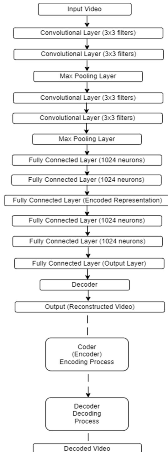
**Figure 5.** CNN network architecture for video encoding and decoding.
