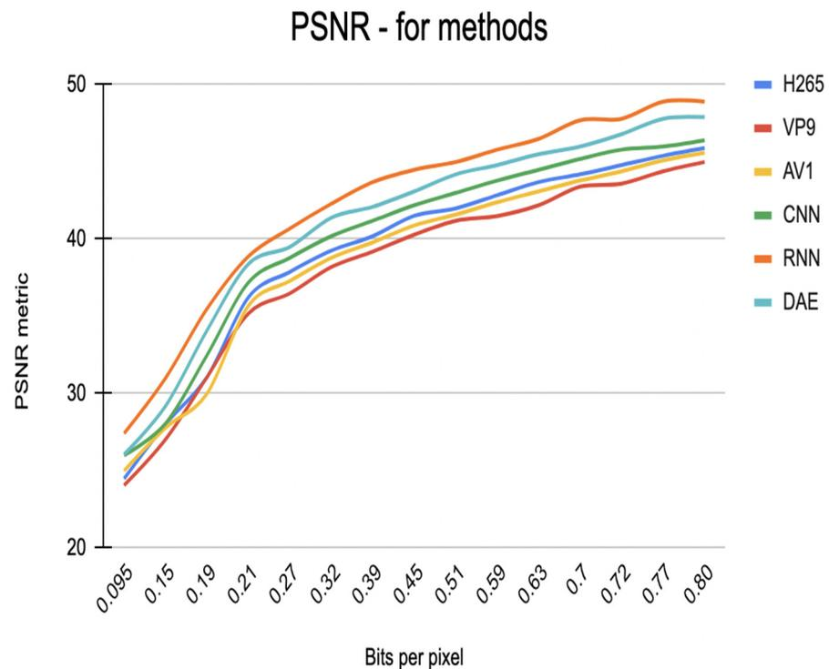
**Figure 11.** Graph of estimation of video compression methods based on PSNR metric.
