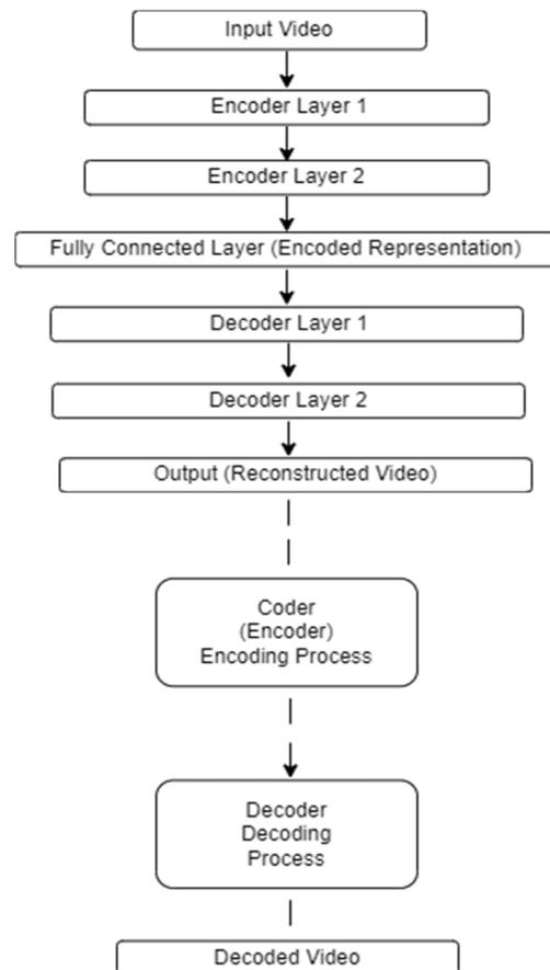
**Figure 9.** The DAE architecture with the encoder–decoder structure.
