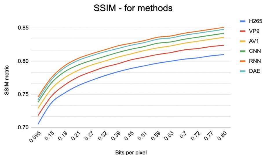
**Figure 12.** Graph of evaluation of video compression methods based on SSIM metric.
