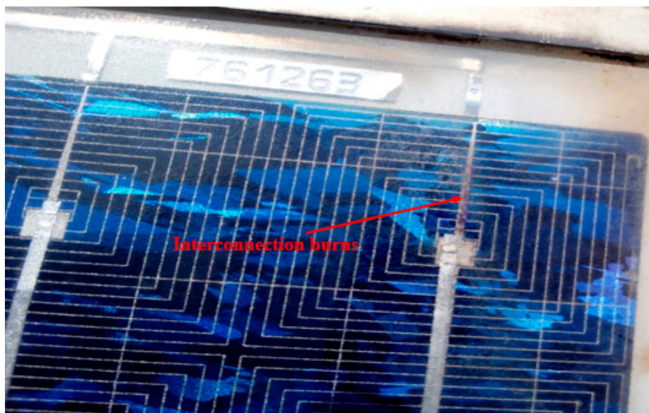
Figure 6. Module 10, indicating interconnection burns.
