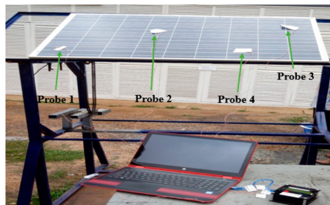
Figure 4. Setup for comparison of IR imager and temperature probes.
