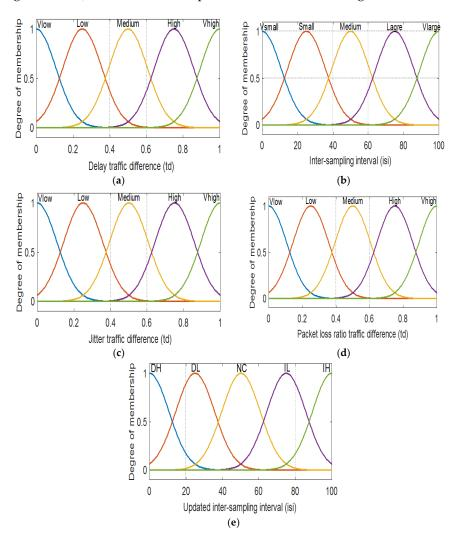
**Figure 7.** Membership functions for (**a**–**c**) the Euclidean distance sets for delay, jitter, and percentage packet loss ratio; (**d**) inter-sampling interval; and (**e**) the updated inter-sampling interval.
