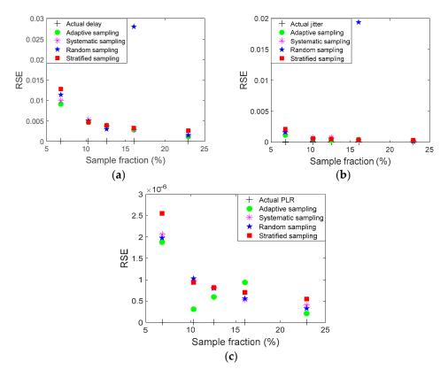
**Figure 11.** Comparisons of RSE of (a) delay, (b) jitter, and (c) PLR between the developed technique and nonadaptive methods.
