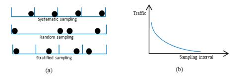
**Figure 1.** An illustration of sampling techniques: (a) Nonadaptive sampling; (b) The concept of adaptive sampling [12].
