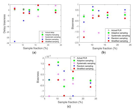
**Figure 10.** Comparisons of biasness of (a) delay, (b) jitter, and (c) %PLR between the developed technique and nonadaptive methods.
