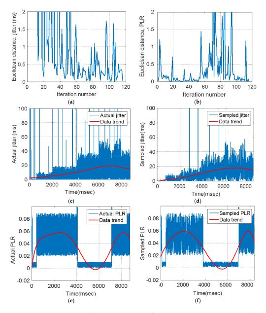
**Figure 9.** Typical results obtained from the developed adaptive technique: (a) measured Euclidean distance for jitter, (b) measured Euclidean distance for packet loss, (c) original traffic jitter, (d) sampled traffic percentage jitter, (e) original traffic packet loss ratio, and (f) sampled traffic packet loss ratio.
