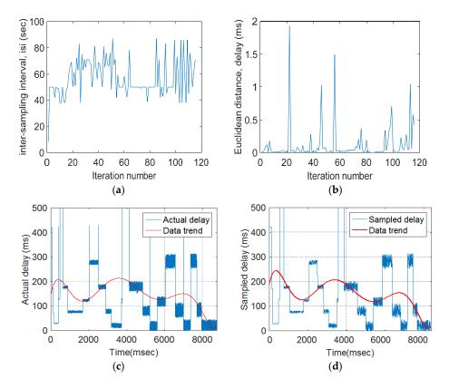
**Figure 8.** Typical results obtained from the developed adaptive technique: (a) FIS output for the inter-sampling interval (*isi*), (b) the Euclidean distance for delay, (c) original traffic delay, and (d) sampled traffic delay.
