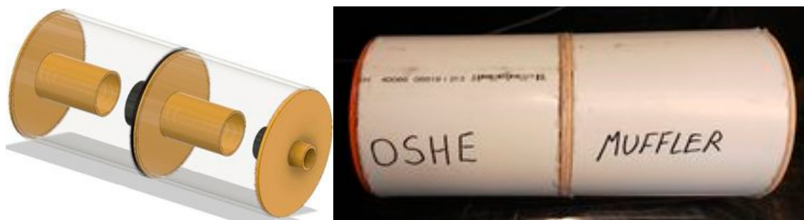
Figure 9. Comparison between computer aided design (CAD) of chamber and finished expansion chamber.
