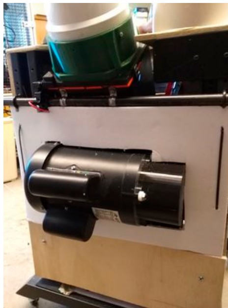
Figure 8. Granulator panel gaps filled with sound proofing material.
