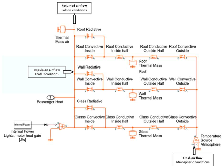
Figure 5. Model of the cabin thermal networking.
