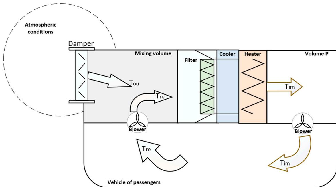
Figure 8. Ventilation system, circulation of air flow.
