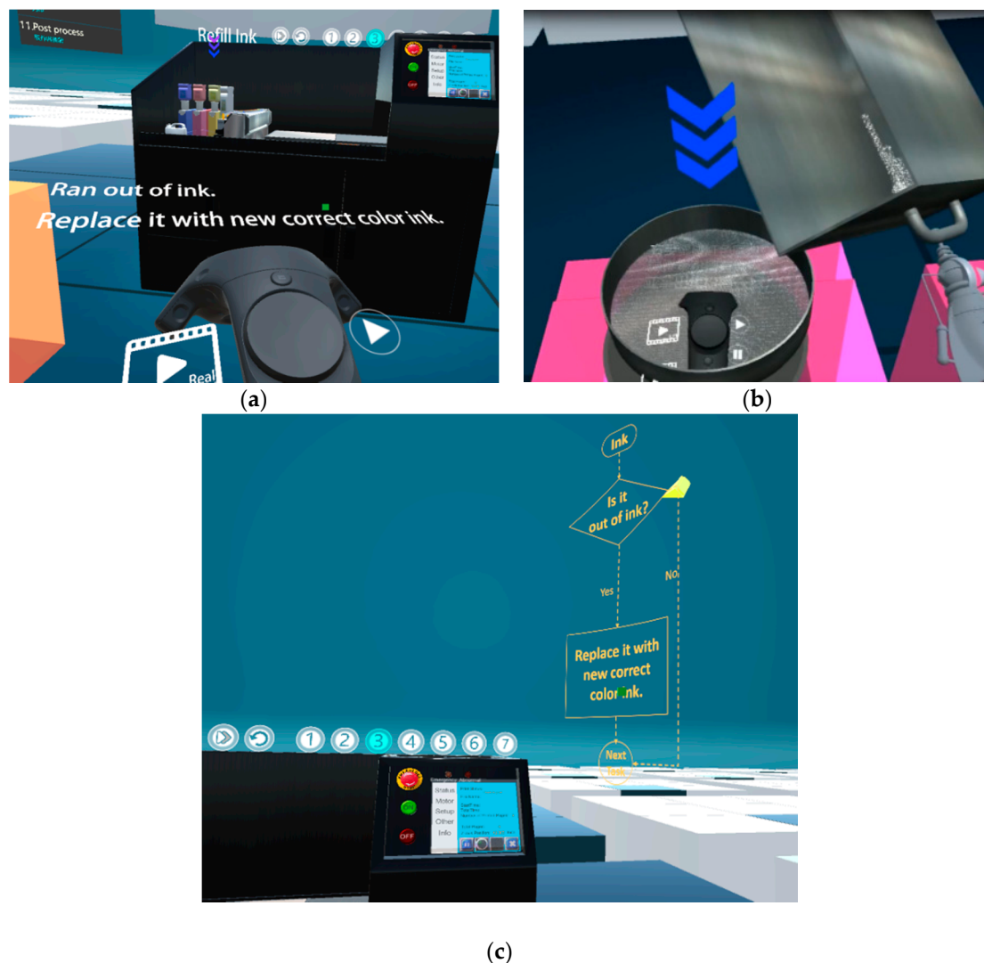
Figure 6. The visual hint information of the 3DP Training Virtual Laboratory: (a) text hint information corresponding to certain work presented above the left-hand controller; (b) the blue arrow showing visual hint information, pointing out the current interaction position/target object; (c) the yellow arrow showing visual hints, pointing out the current progress corresponding to the workflow chart of a certain task.
