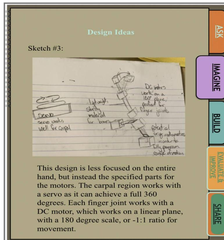
**Figure 1.** Student’s sketch and design idea for mechanical hand.
