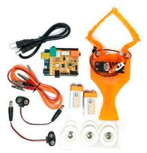
Figure 1. The gripper bundle with the muscle SpikerShield [62].
