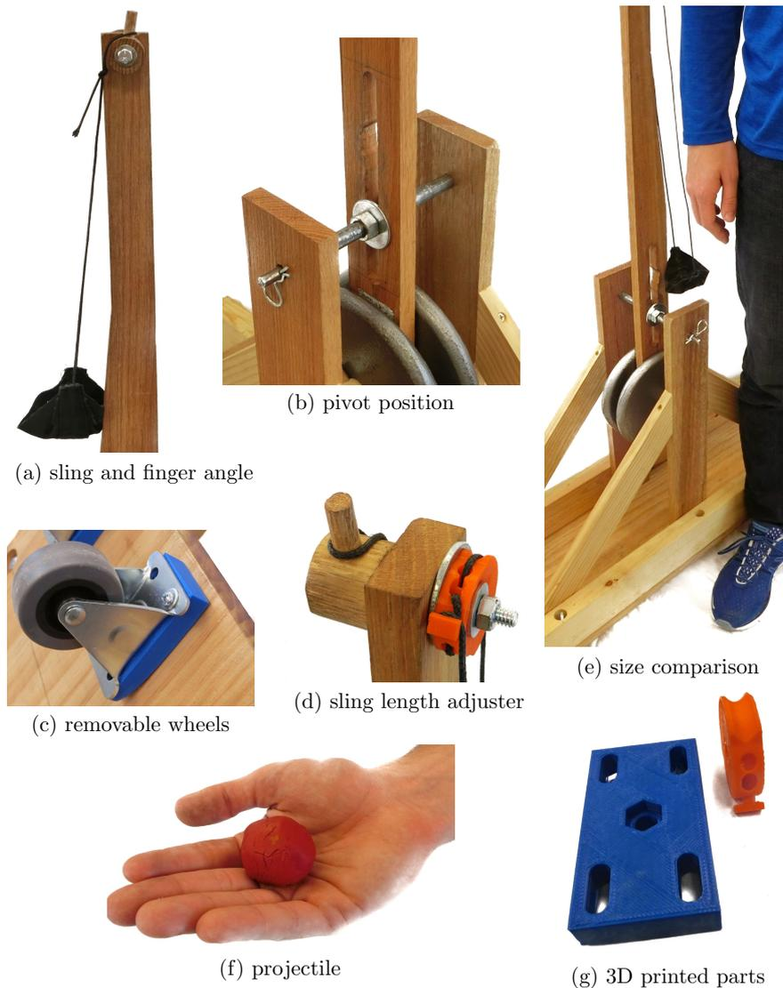
**Figure 6.** Photographs of trebuchet components.
