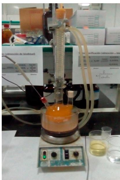
**Figure 6.** Small-scale reactor for transesterification (for high-school students).
