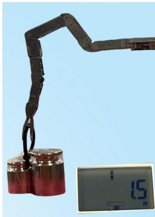
**Figure 11.** Manipulator with effect load of 1.5 (newton and 0.15 kg with down and uploaded).
