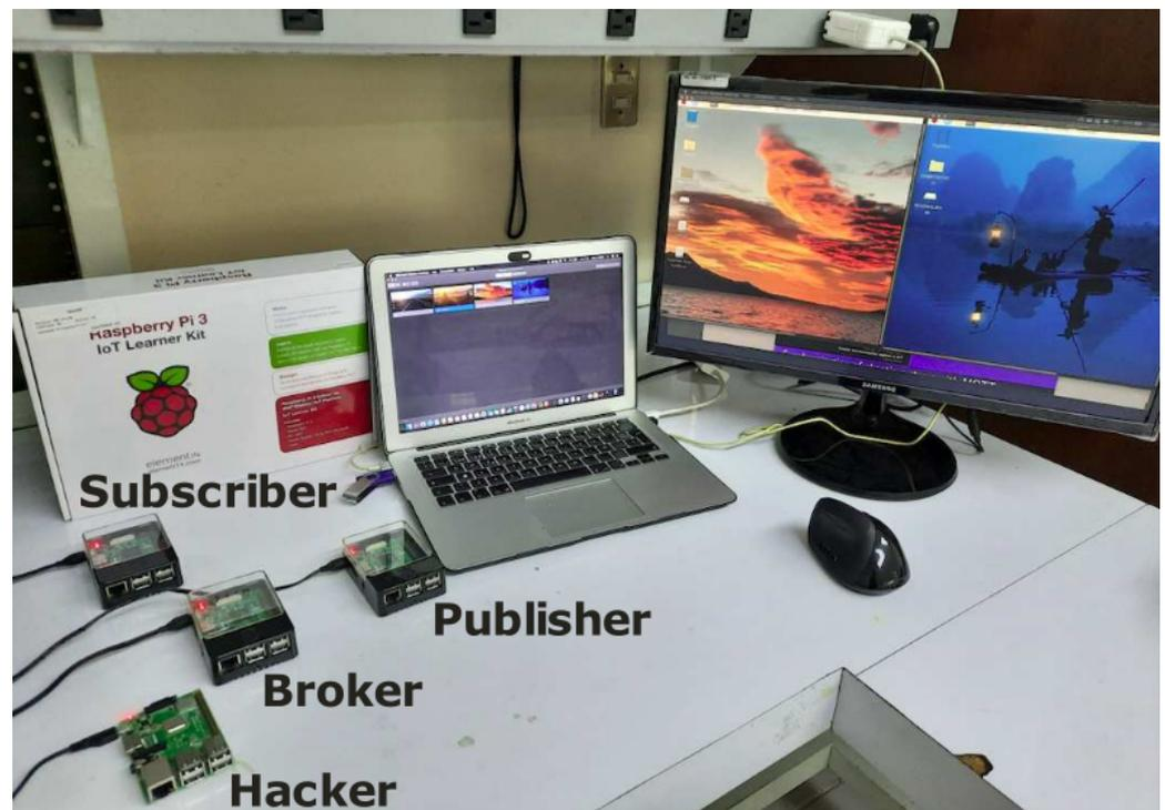
Figure 12. Physical realization of the secure communication system on MQTT for IoT protocol using RPis.
