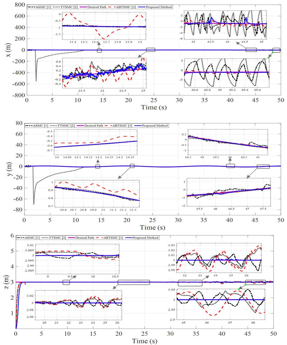
Figure 3. Quadrotor position under 40% sinusoidal fault to actuators 2 and 3.
