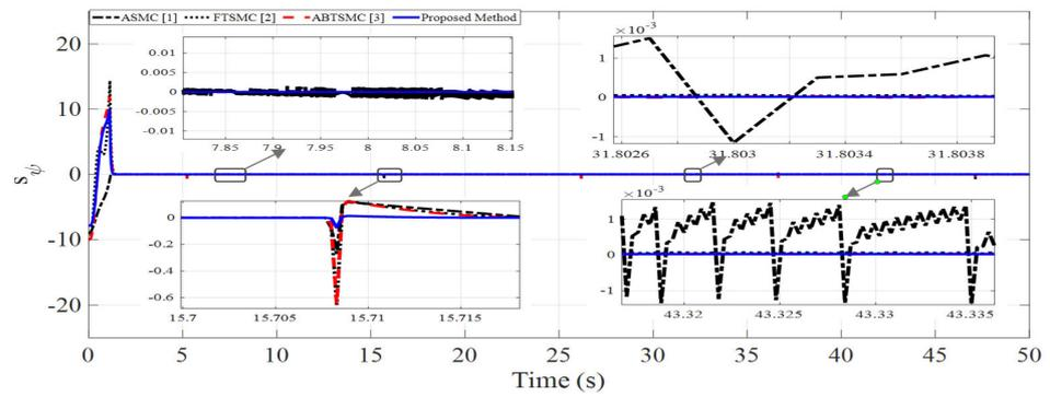
Figure 2. Sliding surface under 40% sinusoidal fault to actuators 2 and 3.
