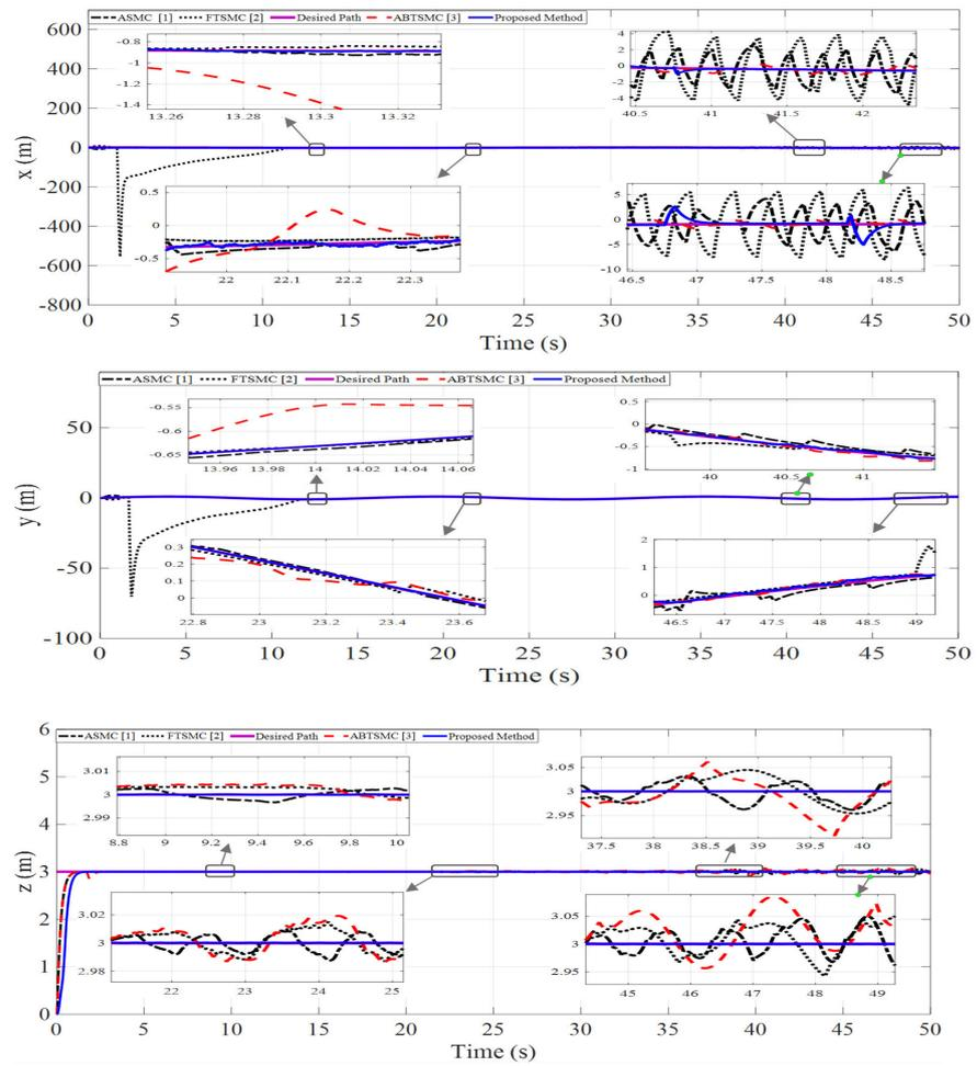
Figure 6. Quadrotor position under 50% step fault to actuators 1 and 2.
