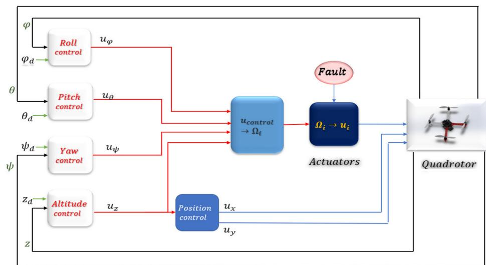
Figure 1. The control scheme of the quadrotor.
