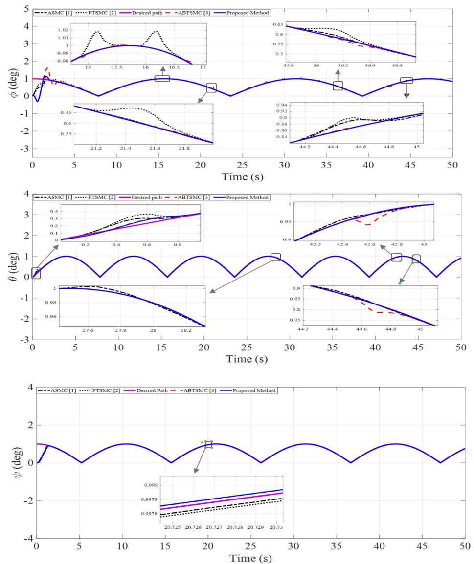
**Figure 4.** Quadrotor attitude under 40% sinusoidal fault in actuators 2 and 3.
