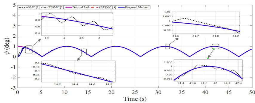
Figure 7. Quadrotor attitude under 50% step fault to actuator 1 and 2.
