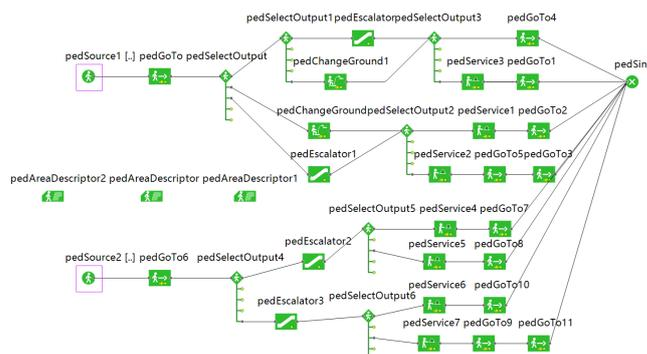
Figure 8. Background operation logic of pedestrian evacuation.
