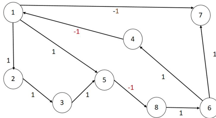
Figure 2. Structurally balanced directed signed graph of eight vertices.
