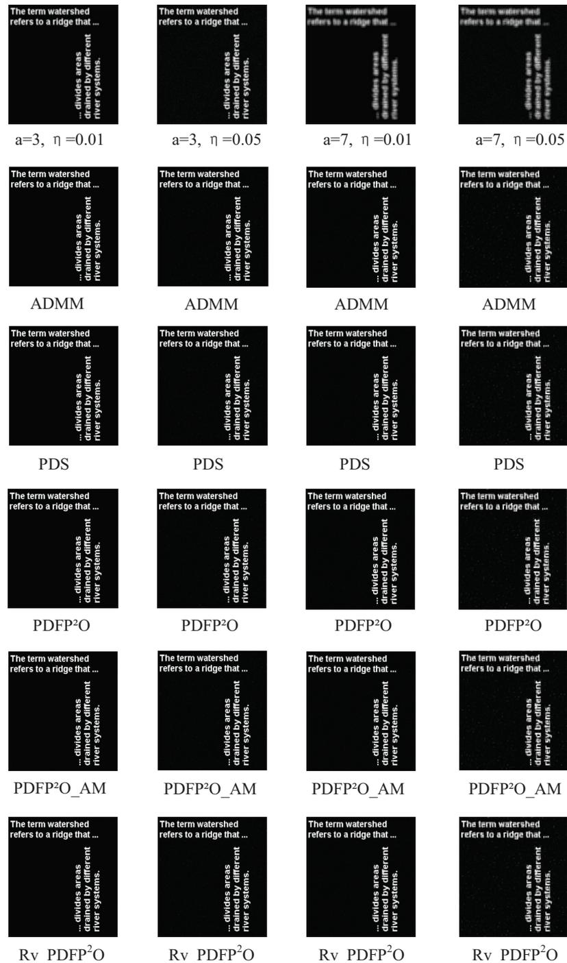
**Figure 2.** These are the “Text” images: **Row 1:** the blurry and noisy images, **Row 2:** the images restored by ADMM, **Row 3:** the images restored by PDS, **Row 4:** the images restored by PDFP<sup>2</sup>O, **Row 5:** the images restored by PDFP<sup>2</sup>O\_AM, and **Row 6:** the images restored by Rv\_PDFP<sup>2</sup>O.
