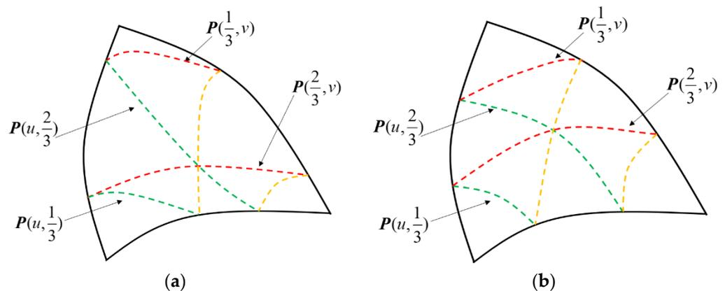
**Figure 1.** Different parameterizations have different iso-parametric curve distributions: (a) poor and (b) good parameterization.
