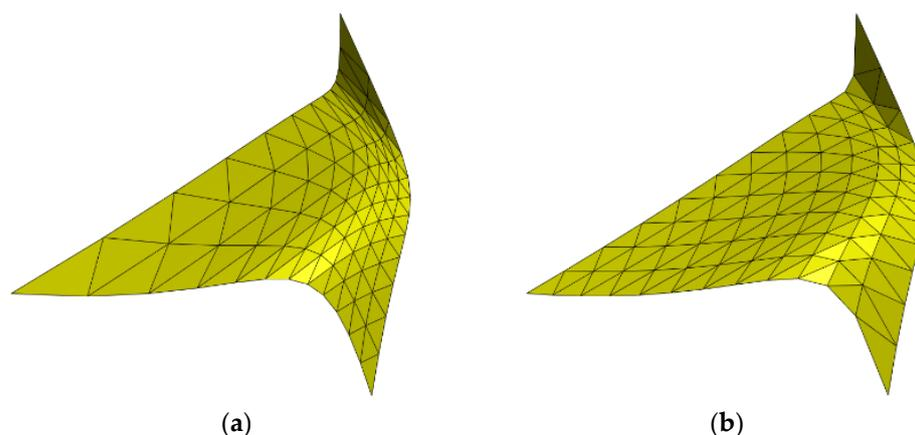
**Figure 4.** Equiareal parameterization with  $\alpha = 0.30$  and  $\beta = 0.36$ . (a) Original surface with  $e = 22.15$ . (b) Resultant surface with  $e(\alpha, \beta) = 10.90$ .
