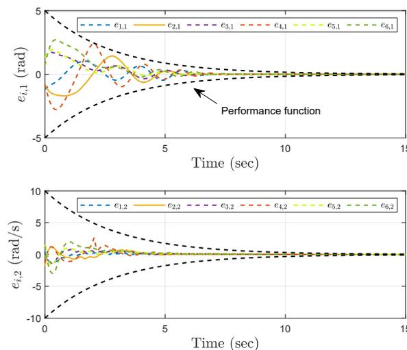
Figure 4. Trajectories of the errors  $e_{i,1}$  and  $e_{i,2}$  under the event–triggered control.
