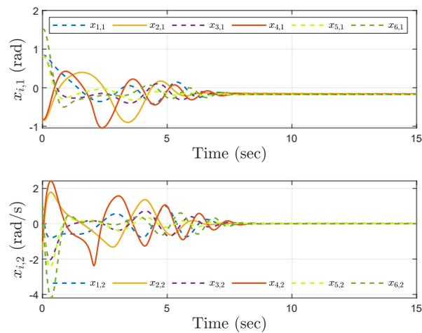
Figure 11. Trajectories of the angles  $x_{i,1}$  and the velocities  $x_{i,2}$  under the time-triggered control.
