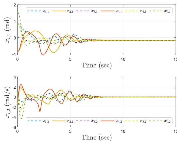
Figure 3. Trajectories of the angles  $x_{i,1}$  and the velocities  $x_{i,2}$  under the event–triggered control.
