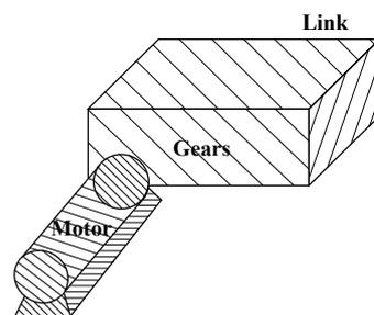
Figure 1. Single-link manipulator.
