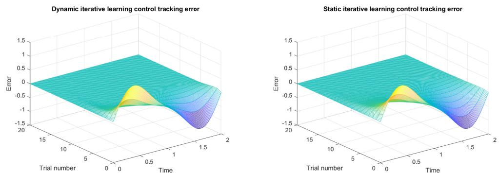
Figure 2. The tracking error curve of ILC at relative degree  $r = 0$ .
