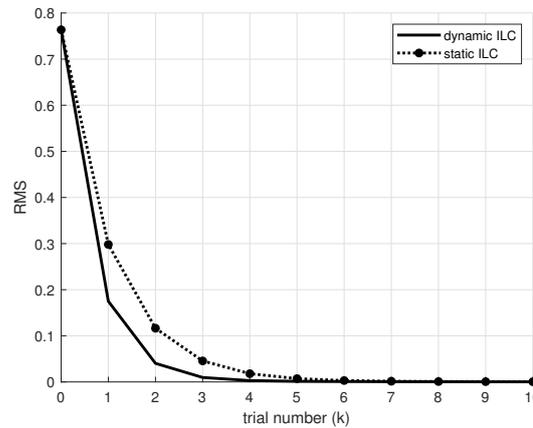
Figure 3. The mean square error trajectory at relative degree  $r = 0$ .
