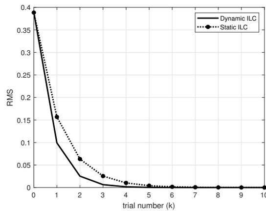
Figure 5. The mean square error trajectory at relative degree  $r = 2$ .
