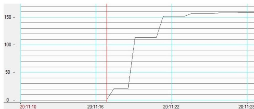
Figure A1. Rotation frequency of the expander rotor according to experimental data.
