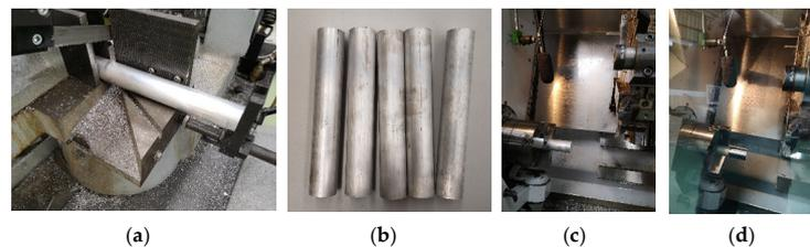
**Figure 4.** Experiment pictures. (a) Parting the stock bars for the experiments. (b) The stocks, ready to be used for the experiments. (c) Machining cabin used in the experiments, with the metal stock bar to be machined. (d) The machined part.
