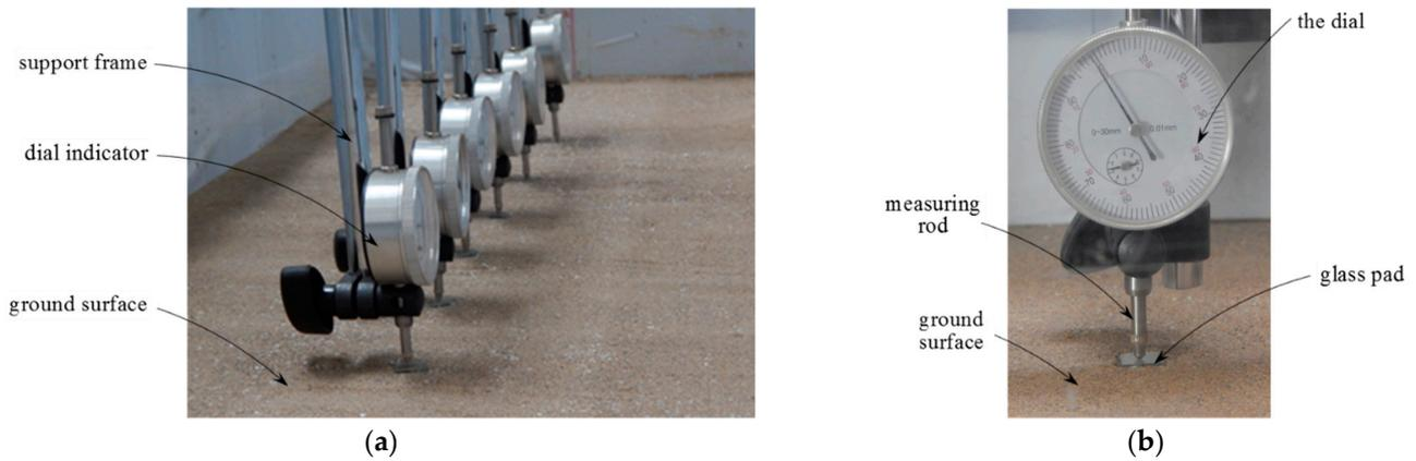
**Figure 5.** Monitoring of the surface settlement. (a) Arrangement of the dial indicator; (b) installation details of the dial indicator.
